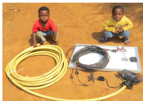
Photograph 2. Complete, entry-level irrigation system using one ZKSJ pump
