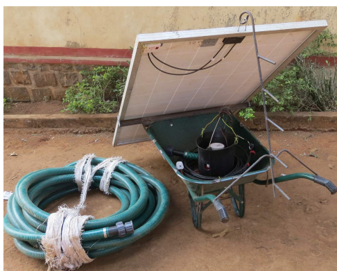
Photograph 3. Complete irrigation system using one Seaflo 3700 pump
