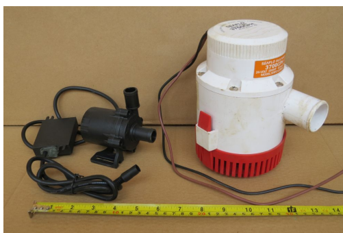
Photograph 1. ZKSJ model DC50B-24130S and Seaflo 3700 pumps
