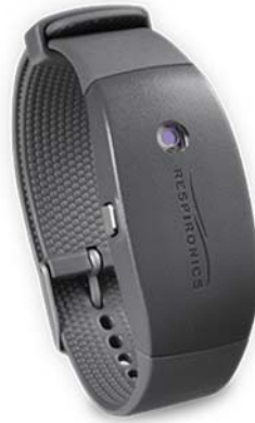
Figure 2.3. Actiwatch 2 device by Phillips Respironics, USA. The device was setup to capture 14 days of data, monitoring activity and photopic light using the inbuilt accelerometer.
