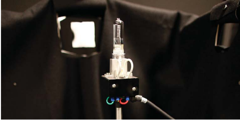
Figure 4.3: Experimental setup for FEL lamps annealing - photography of the lamp mounted in testing post
