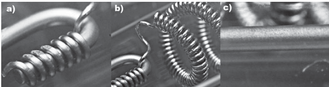
Figure 4.11: Enlargements of filament degradation of Ushio lamp after 96h of annealing: a) and c) filament support b) filament
