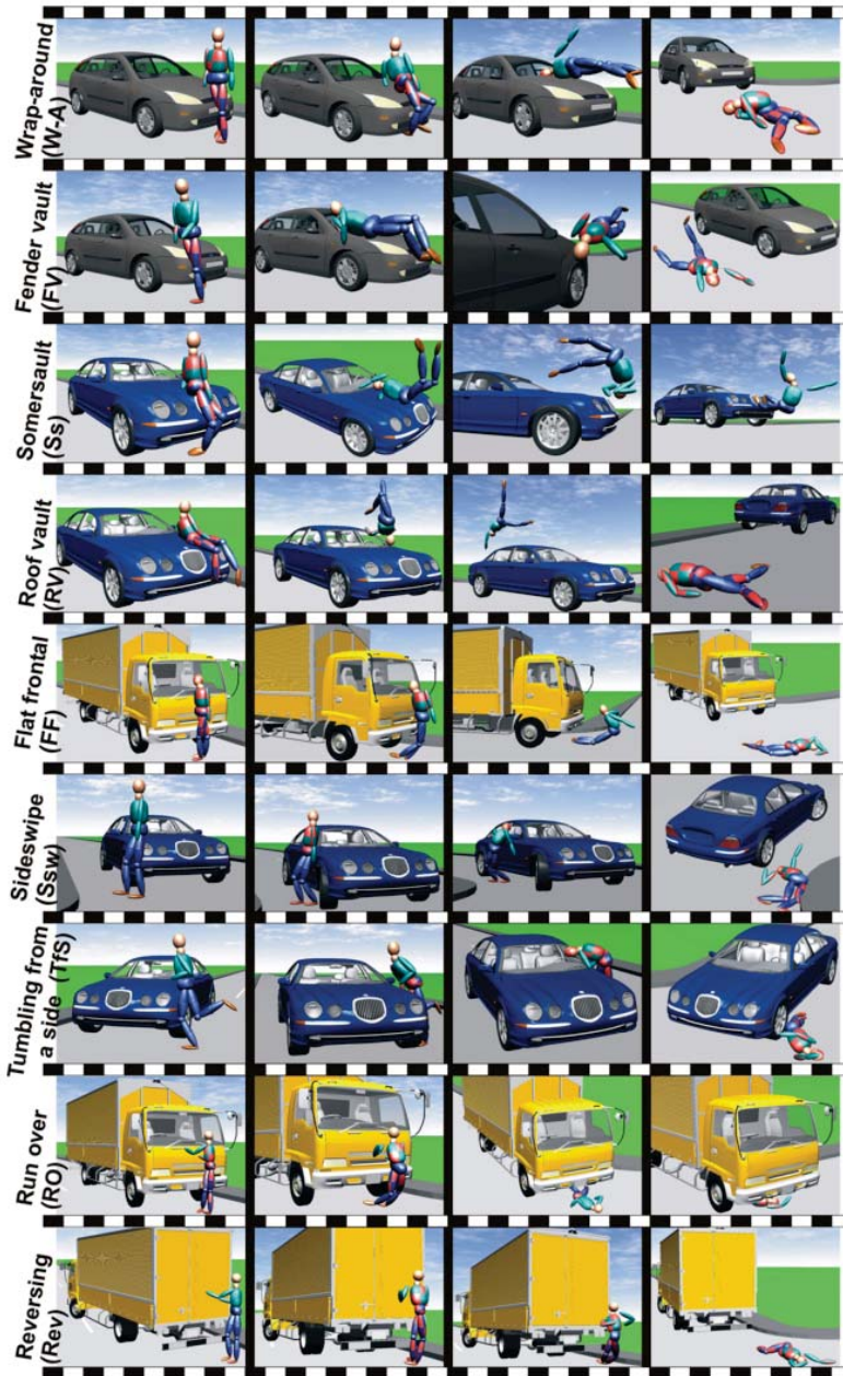
Figure 1: Interaction between vulnerable road user (pedestrian or pedal cyclist) and striking vehicle.
