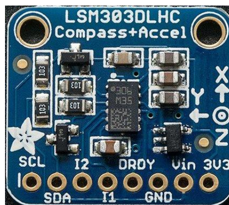
Figure 5.4: LSM303DLHC mounted on Adafruit board
