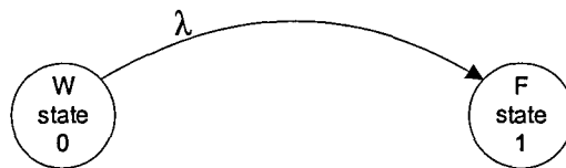
Figure 2.11 Single Non-Repairable Component Markov Transition Diagram
