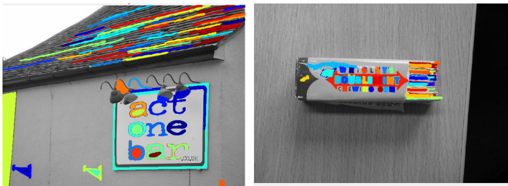
Figure 4.10: The result of using MSER detector
