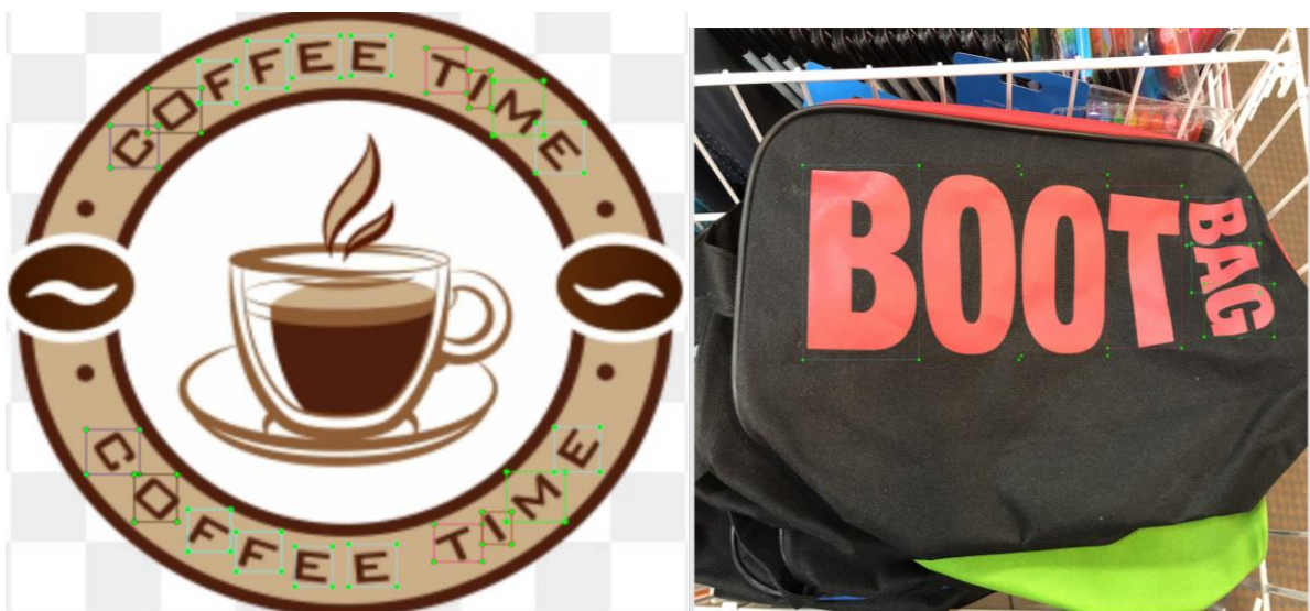
Figure 5.10: Example of annotation of different text orientations (Horizontal, curve, irregular). Word level
