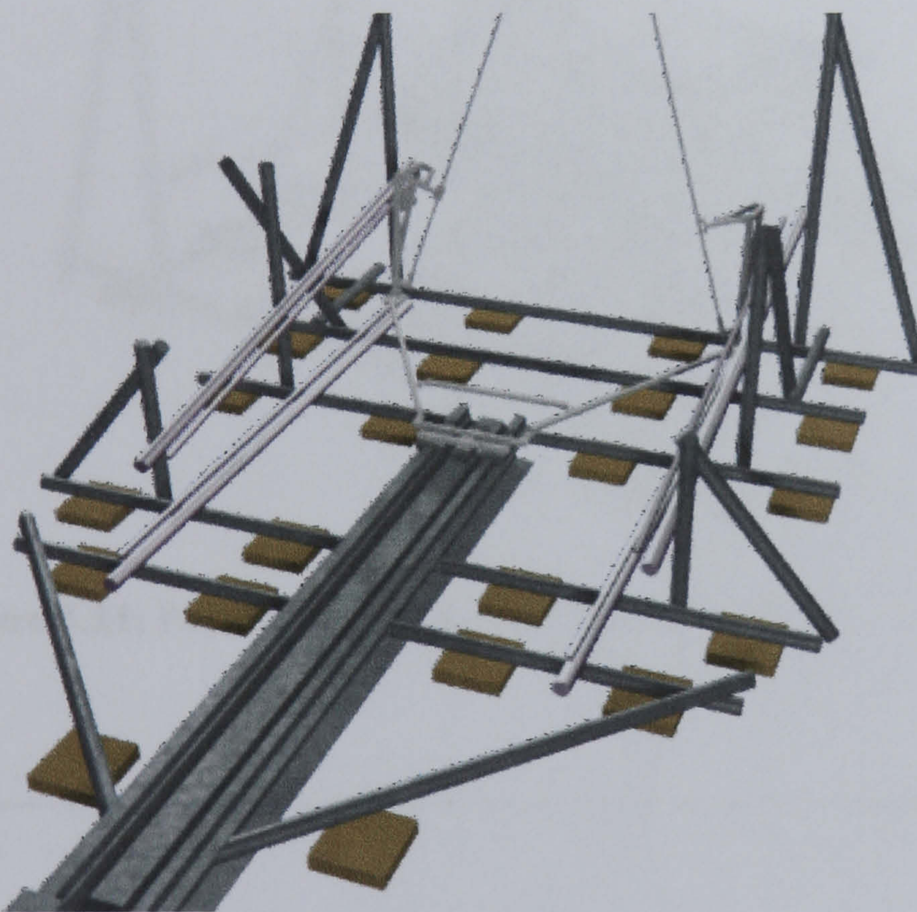
Figure 5.10: Cassettes, triangular linkages, ski poles and A-frame linkage to actuator
