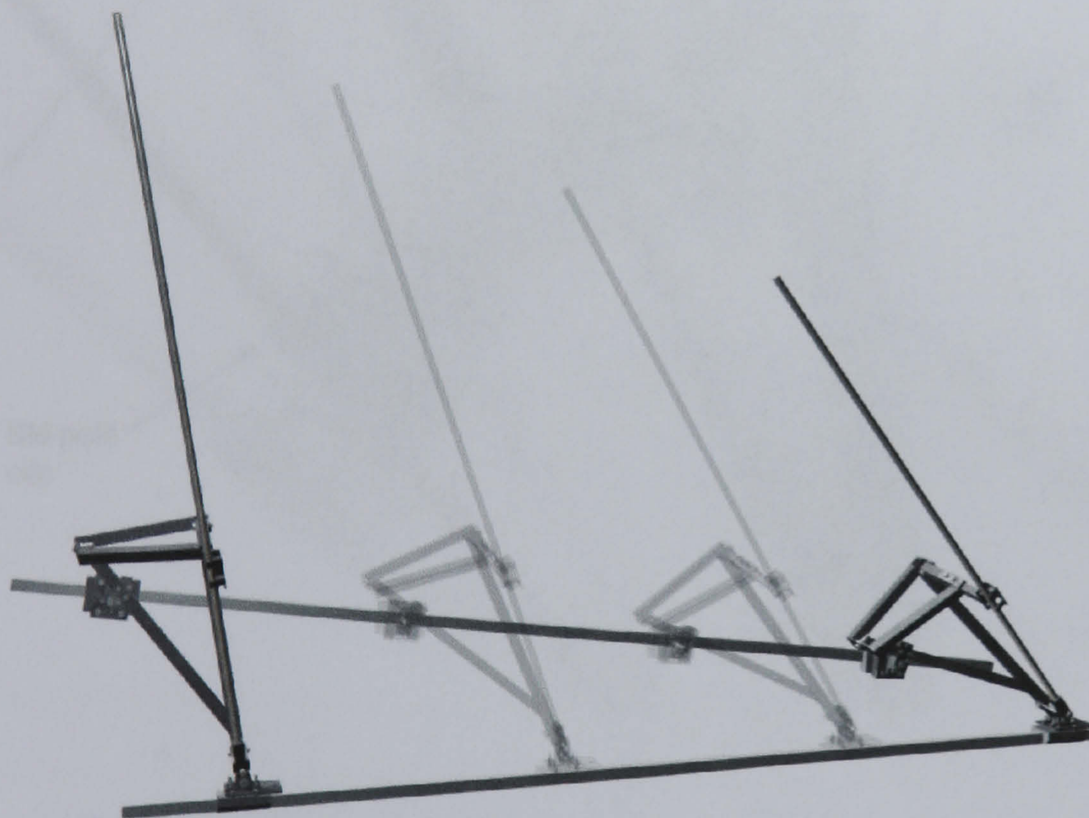
Figure 5.3: Change of pole angle through stroke
