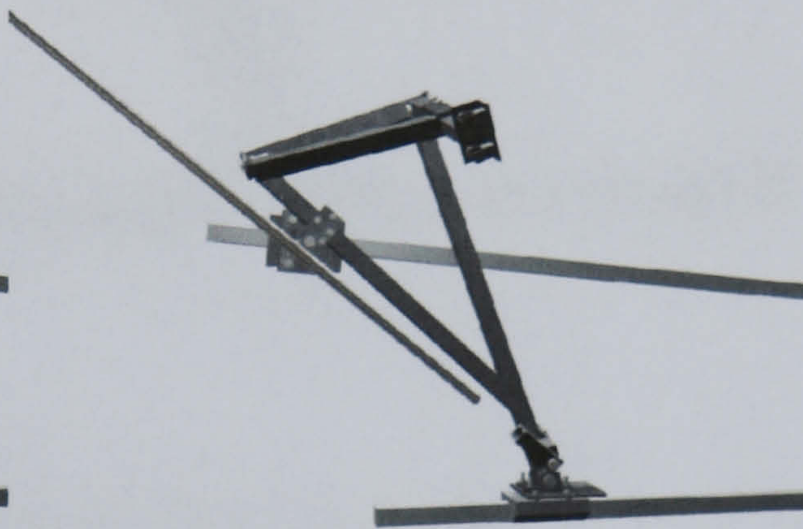
4) Pole pulls free of socket becoming separated from moving parts.
