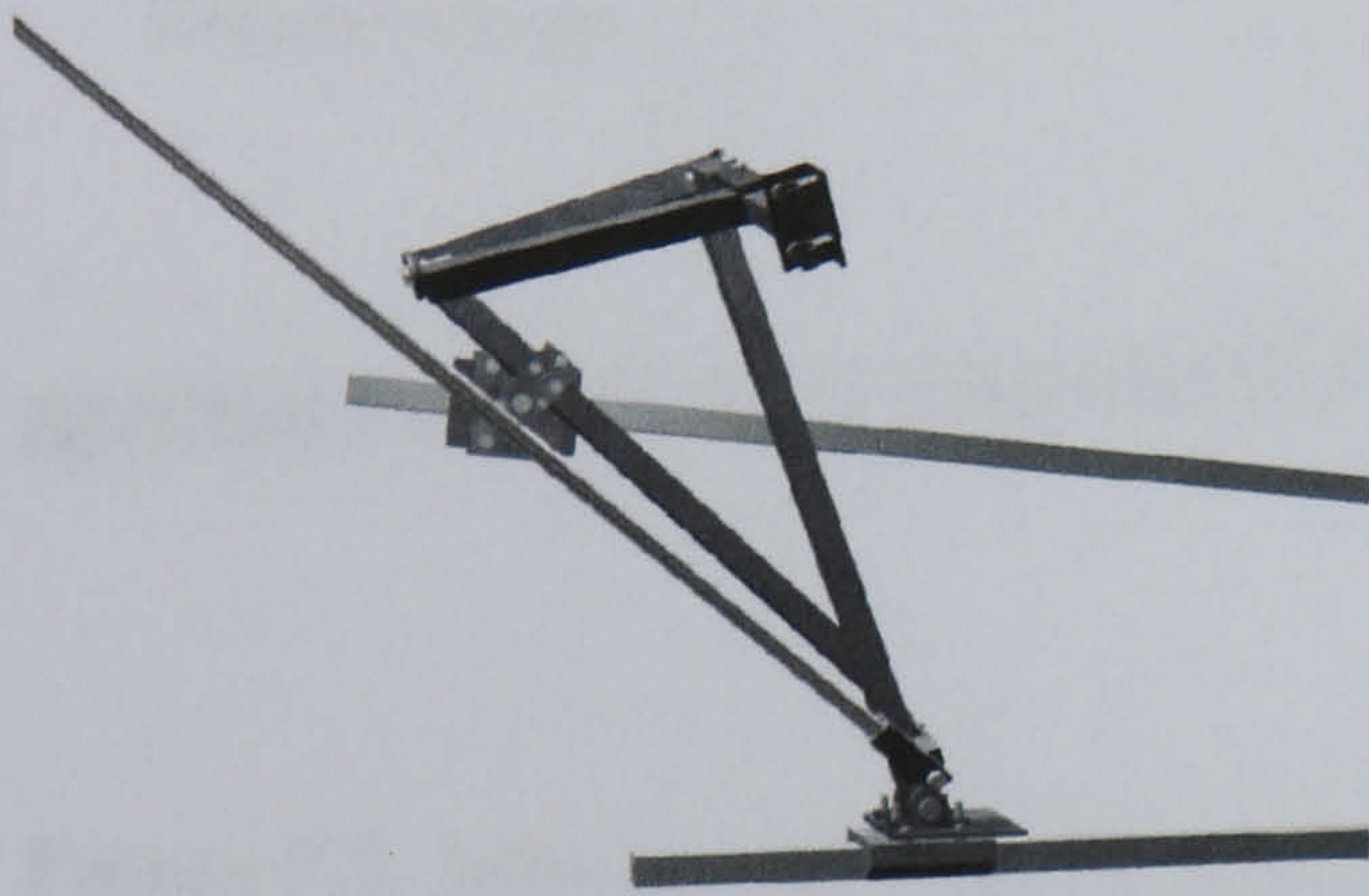
3) Pole rotates forwards in tip socket as moving parts come to a standstill.
