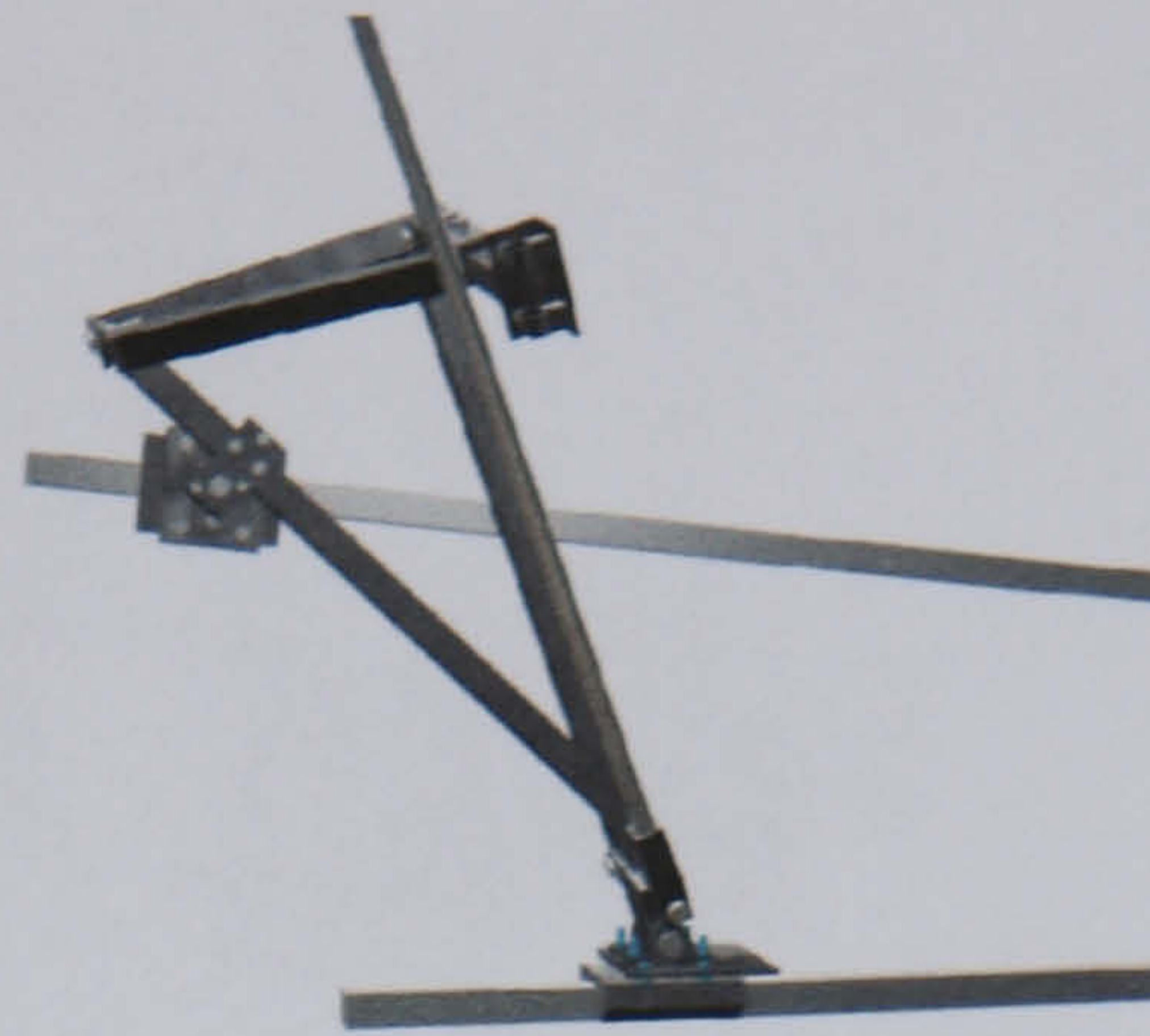
2) Pole becomes unclipped and breaks emergency stop circuit.
