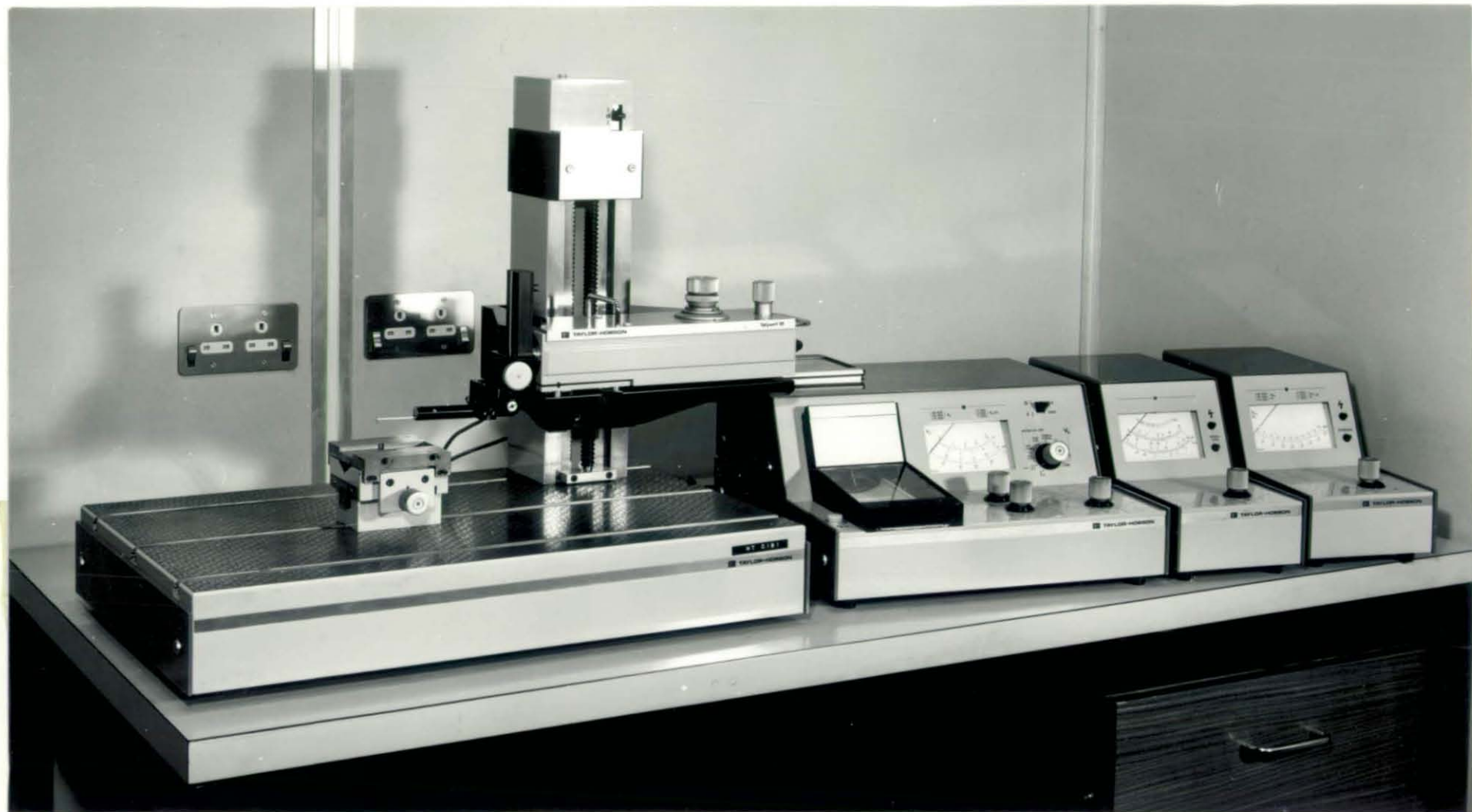
Plate 3.7. Taylor-Hobson Talysurf 10 Roughness Measurement Device
