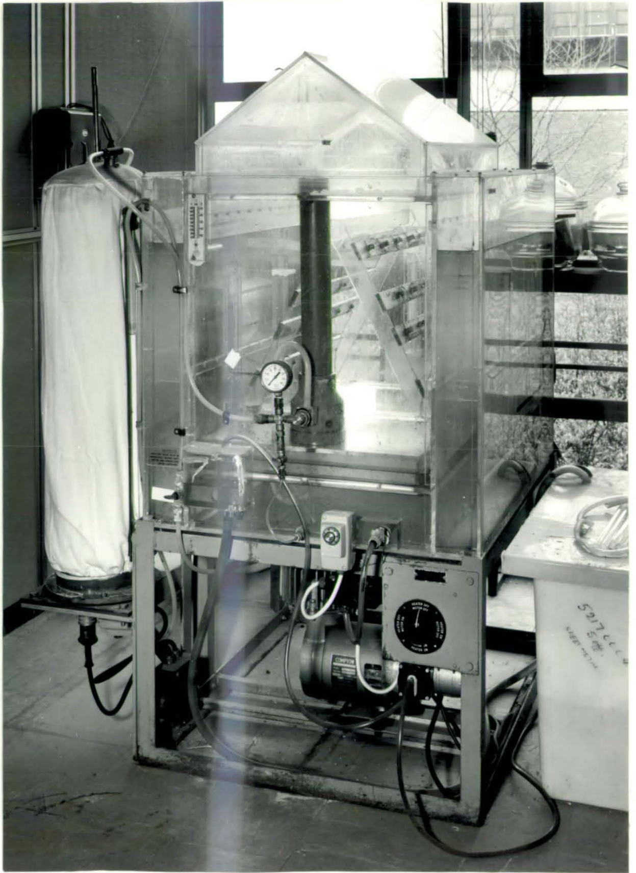
Plate 3.8. Salt-Spray Test Chamber
