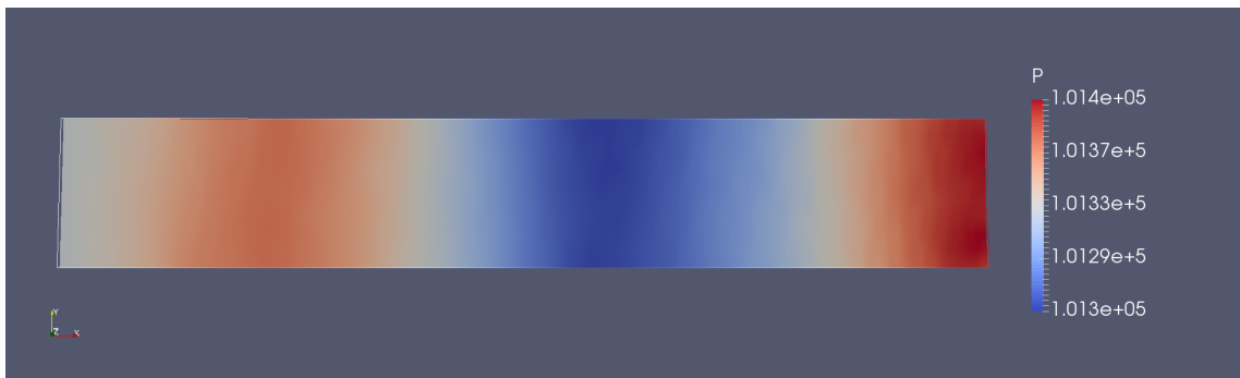
Figure 5.3: Snapshot of pressure field assuming a pressure node at the upstream (left hand side) boundary.
