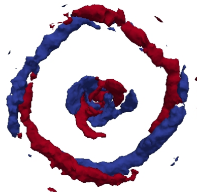
(d) The heat release component for the 2nd most energetic POD mode.
