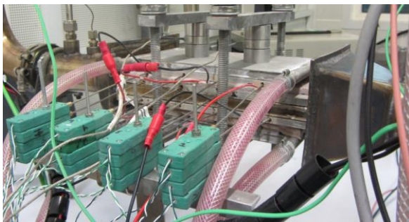
Figure 8. TEG installed in the EGR path for engine test
