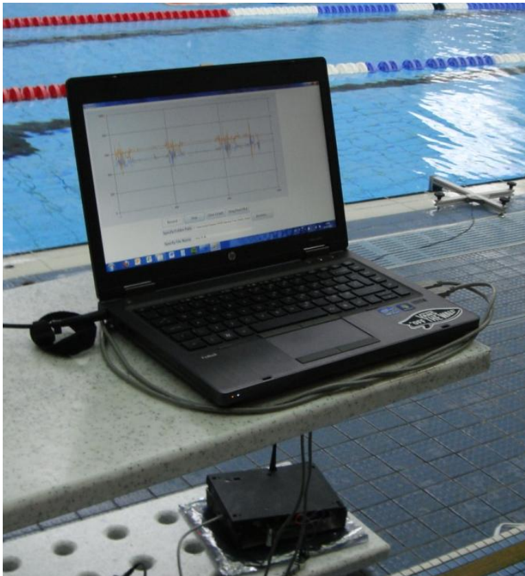
Figure 55: Wireless sensor node (WSN) capture during turn testing
