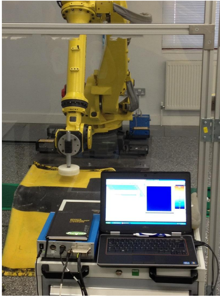
Figure 61: Pressure mat validation using a robotic arm and force platform
