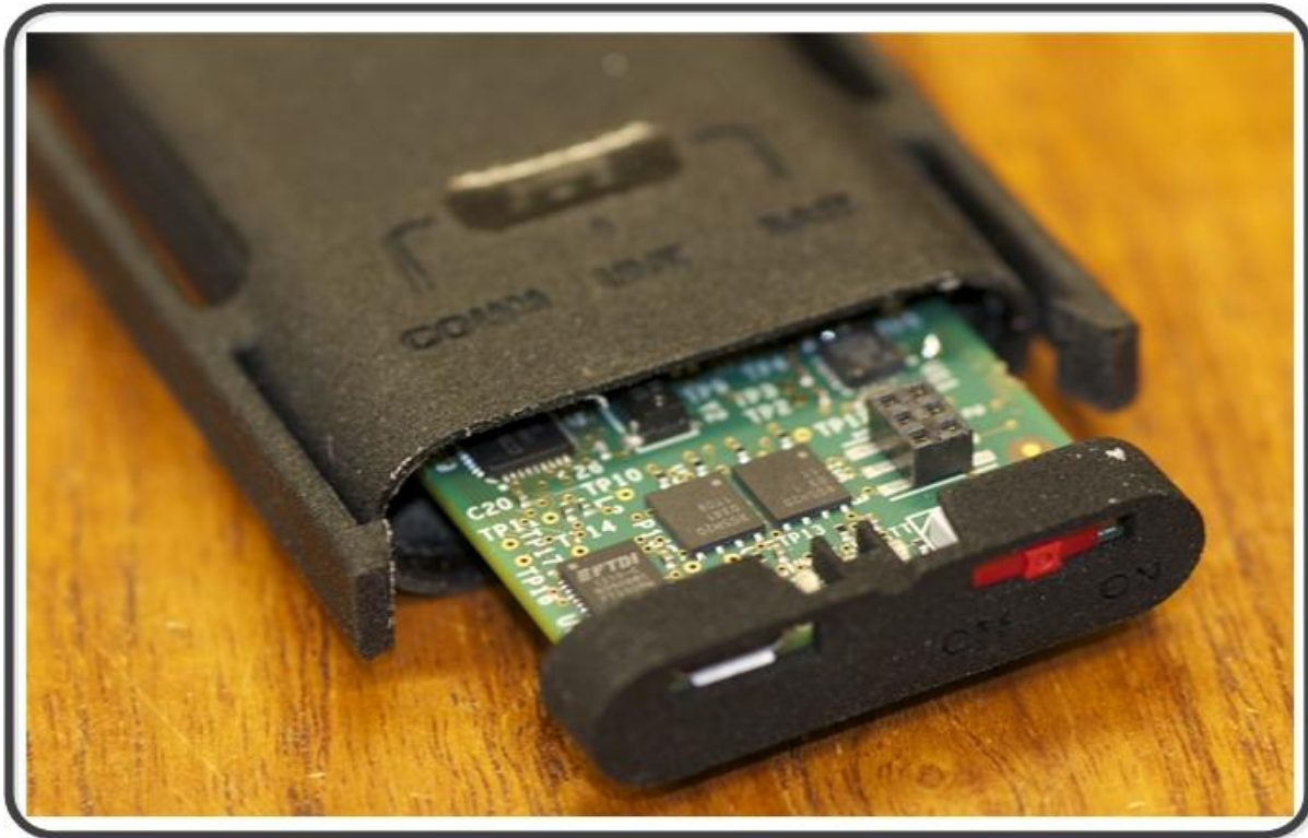
Figure 30: Contents of the wireless sensor node (WSN) in March 2013.
