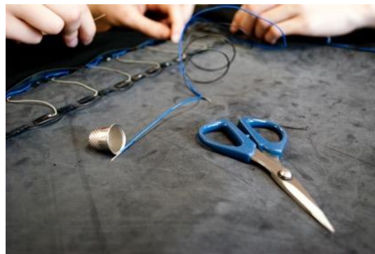
Fig. 8. The wiring of the solar cells on the inside of the Solar Dress
