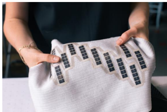
Fig. 9. Solar cells combined with printed electronics, laminated to textile
