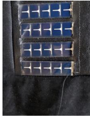
Fig. 7. Solar cells fixated inside leather
