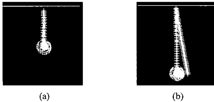
Fig. 5.5. Bounce of the cue ball from the cushion, the ball location depicts its position as it approached the rail (at 120 fps frame rate)
