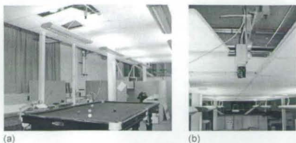
Fig. 1. Snooker table and ceiling-mounted machine vision camera in the mechatronics laboratory. Note the headspace and the vertical mount of the camera to look perpendicularly down at the table.
