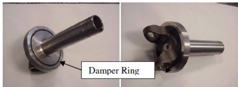
Figure 2.11- View of slip yoke damper ring (after Lee, 2007)
