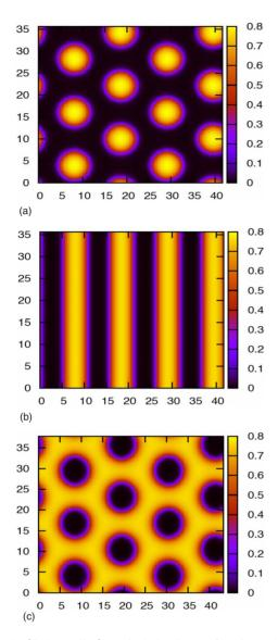
FIG. 2. (Color online) Typical density profiles in each of the microphase separated phases. These profiles are for the temperature  $k_BT/\epsilon=0.15$  and the average densities are  $\rho\sigma^2=0.2$ , 0.35, and 0.5 in the cluster, stripe, and bubble phases, respectively. The *x* and *y* axes are in units of  $\sigma$ .
