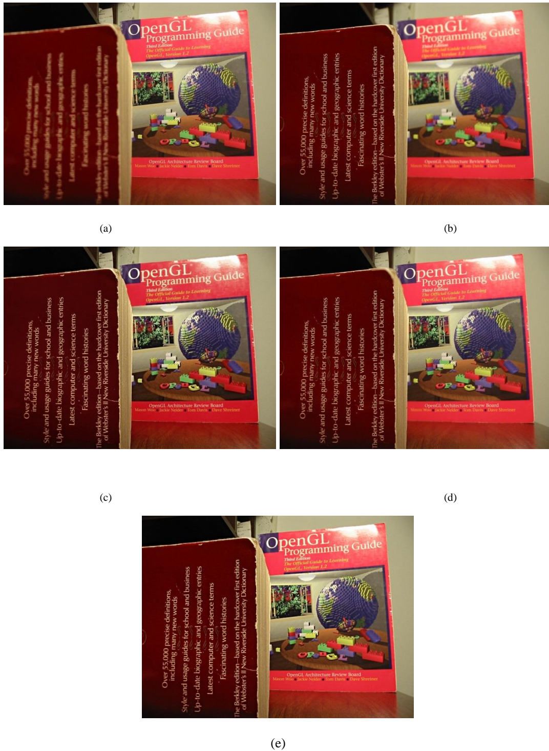
Figure 5.15: Multi-focus image fusion comparison: (a) and (b) show the original set of multi-focus images. (c) is the result of the image fused with the algorithm proposed. (d) is the resulting fused images using a LP fusion approach; and in (e) a spatial frequency fusion approach is used.
