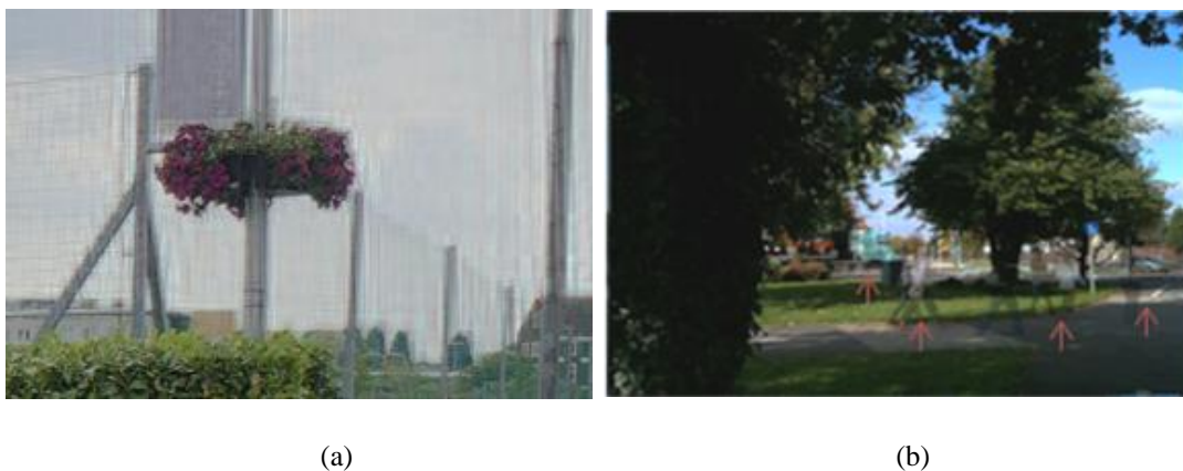
Figure 5.6: (a) Fusion artefacts that appear in a fused image (150 % zoom) when using a WCBT fusion as in section 5.4.2.1. Visible artefacts: blockiness, loss of resolution, chromatic aberrations effect, and hazy appearance. b) Image with a ghosting effect (indicated by the arrows).
