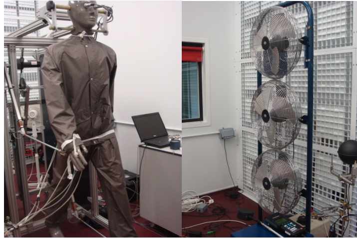
Fig. 4 The test setup of the manikin and the fans used for air movement. The left picture shows the neck and bottom opening closed.
