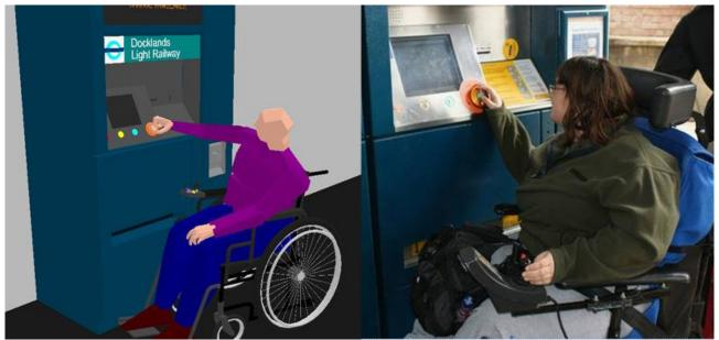
Figure 4: HADRIAN performing a task analysis in SAMMIE and the equivalent in the real world
