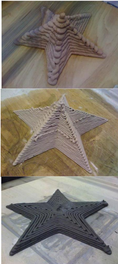
Figure 6: Printing examples of two resolutions. Left: 22 by 15mm using gypsum. Middle and Right: 9 by 6mm using gypsum and cement-based materials.
