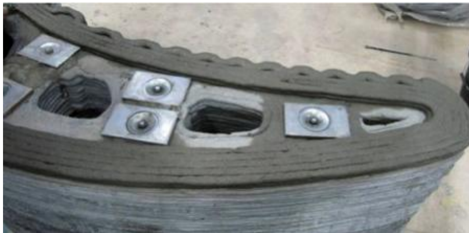
Figure 10: Internal structure including functional voids and reinforcement.
