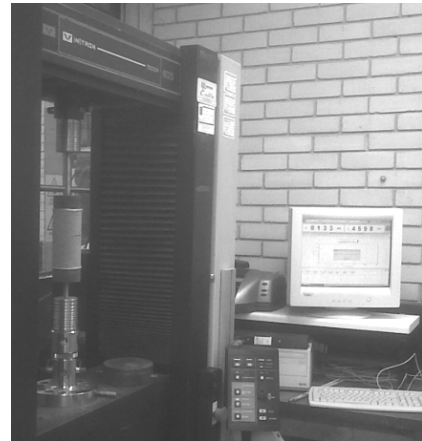
a) Coring six 58x120 mm cylinder specimens from a beam bond component b) Testing tensile bond strength
