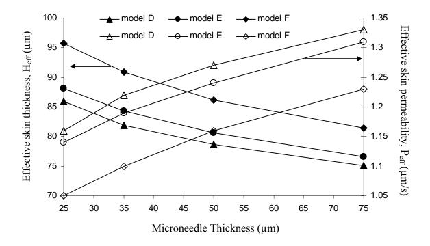
$\label{eq:Figure 6.} Figure 6. Influence of microneedle thickness of insulin coated microneedles models on effective skin thickness $H_{eff}$ (solid markers) and effective skin permeability $P_{eff}$ (blank markers).$
