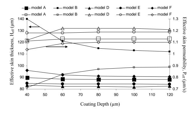
Figure 7. Influence of microneedle coating depth of insulin for various microneedles models on effective skin thickness  $H_{\text{eff}}$  (solid markers) and effective skin permeability  $P_{\text{eff}}$  (blank markers).
