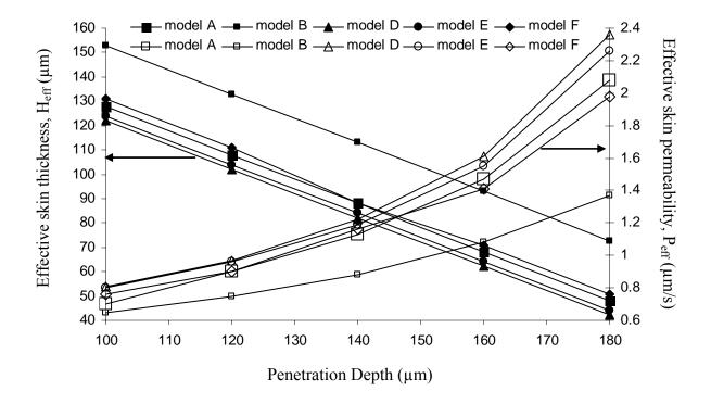
Figure 4. Influence of the changing penetration depth of various microneedles models, coated with insulin, on effective skin thickness  $H_{\text{eff}}$  (solid markers) and effective skin permeability  $P_{\text{eff}}$  (blank markers).
