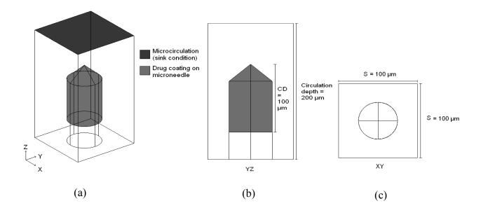
Figure 3. A schematic model for modelling diffusion from a microneedle through the skin: (a) 3D view, (b) side view and (c) top view. CD is the coating depth of drug on the microneedle and S is the width and length of the square element of skin.
