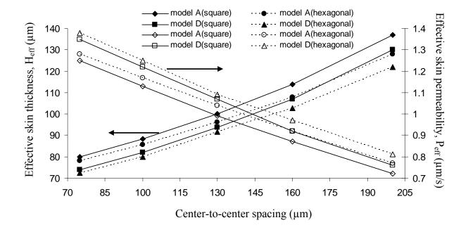
Figure 9. Comparison of the effects of insulin coated microneedle spacing for models A and D for square and hexagonal microneedle patterns on effective skin thickness  $H_{eff}$  (solid markers) and effective skin permeability  $P_{eff}$  (blank markers).
