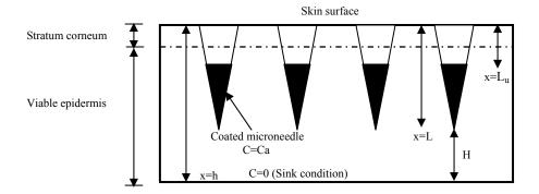
Figure 1. Schematic of coated microneedles for transdermal drug delivery.  $L_u$  is the uncoated microneedle length, L is the total microneedle length, h is the epidermis thickness and H is the thickness of the skin after microneedles have been inserted, i.e., the distance between microneedle tip and the blood micro-circulation.
