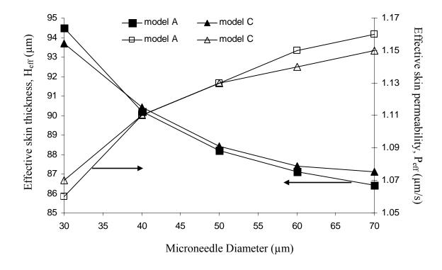
Figure 5. Influence of the microneedle diameter of insulin coated microneedles models on the effective skin thickness  $H_{\text{eff}}$  (solid markers) and effective skin permeability  $P_{\text{eff}}$  (blank markers).
