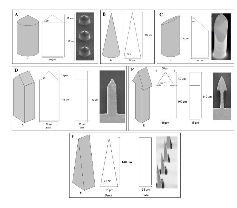
Figure 2. The different microneedles models used for coating drugs. (A) was fabricated by Xie *et al.* (2005), (B) was fabricated by Henry *et al.* (1998), (C) was proposed by McAllister *et al.* (2003), (D) & (E) were fabricated by Gill and Prausnitz (2007) and (F) was fabricated by Martanto *et al.* (2004).
