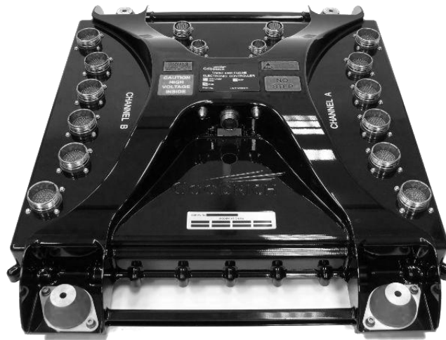
Figure 2.3.2: A typical EEC for a large civil engine. The two redundant channel are clearly marked on the case and physically isolated within the unit. ( figure courtesy of Aero Engine Controls )
