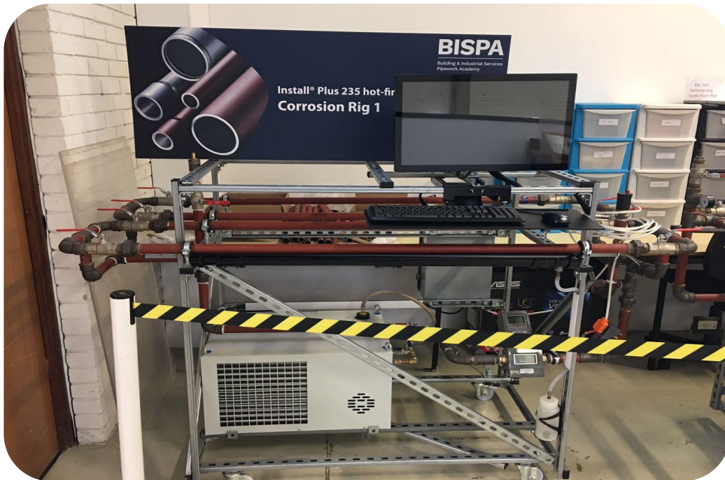
Figure 3.5 BISPA Corrosion Experimental Rig
