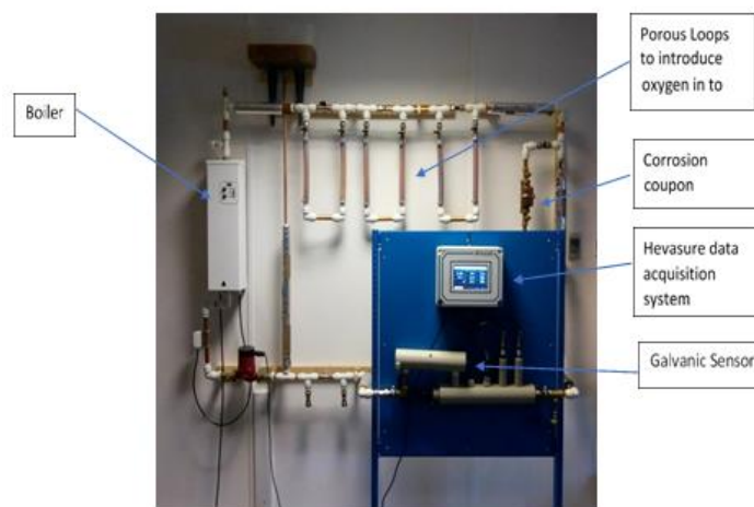
Figure 3.8 Hevasure Corrosion Experimental Rig
