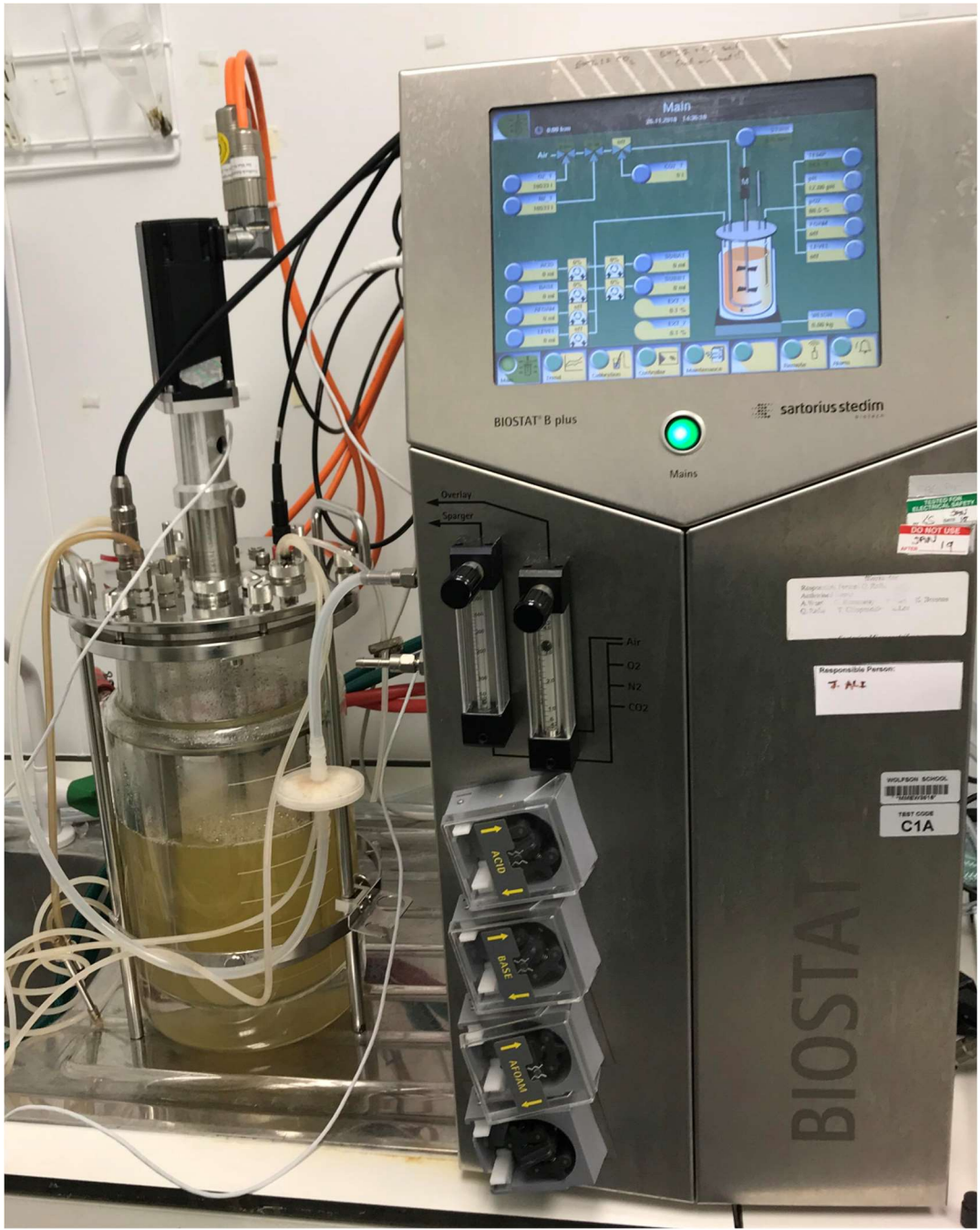
Figure 2.6. An image to show the setup of the 5L bioreactor
