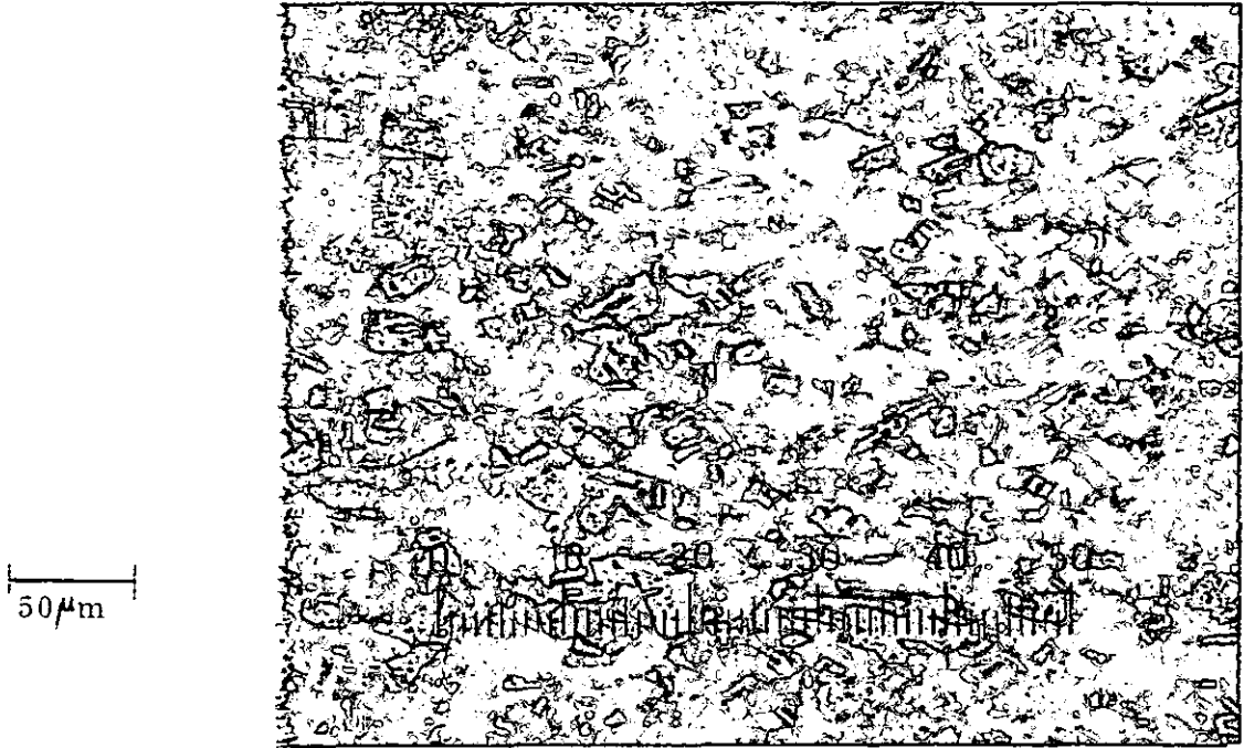
Figure 9.1 Unstrained Compressive Specimen - Annealing Temperature 310°C
