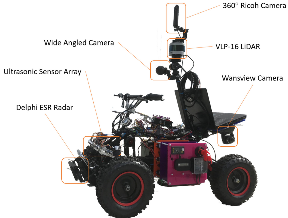
Figure 20: Loughborough University London autonomous platform indicating the location of the range and optical sensors used to collect the LboroLdn AV and LboroLdnHAR datasets. The Kinect sensor, missing from this image, is positioned on the handlebar.
