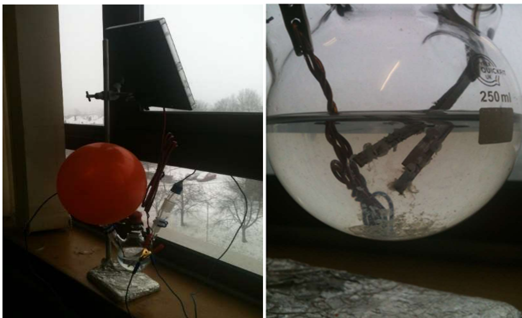
Figure 1.14 Carboxylation of olefins using solar panel. (Buckley B,R.)
