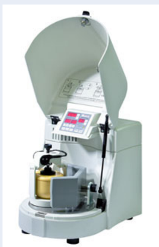
Fig. 3-2. The photograph of Fritsch Pulverisette-6 planetary ball milling machine used in this project.
