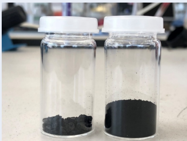
Fig. 5-7. Photos of 100 mg of (left) as-prepared GO and (right) fluffy annealed GO, showing the large volume expansion (almost doubles the apparent volume) upon annealing treatment at 250 °C in argon atmosphere.
