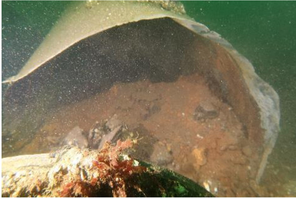
Figure 5: Mine November – end plate ejected by internal overpressure
