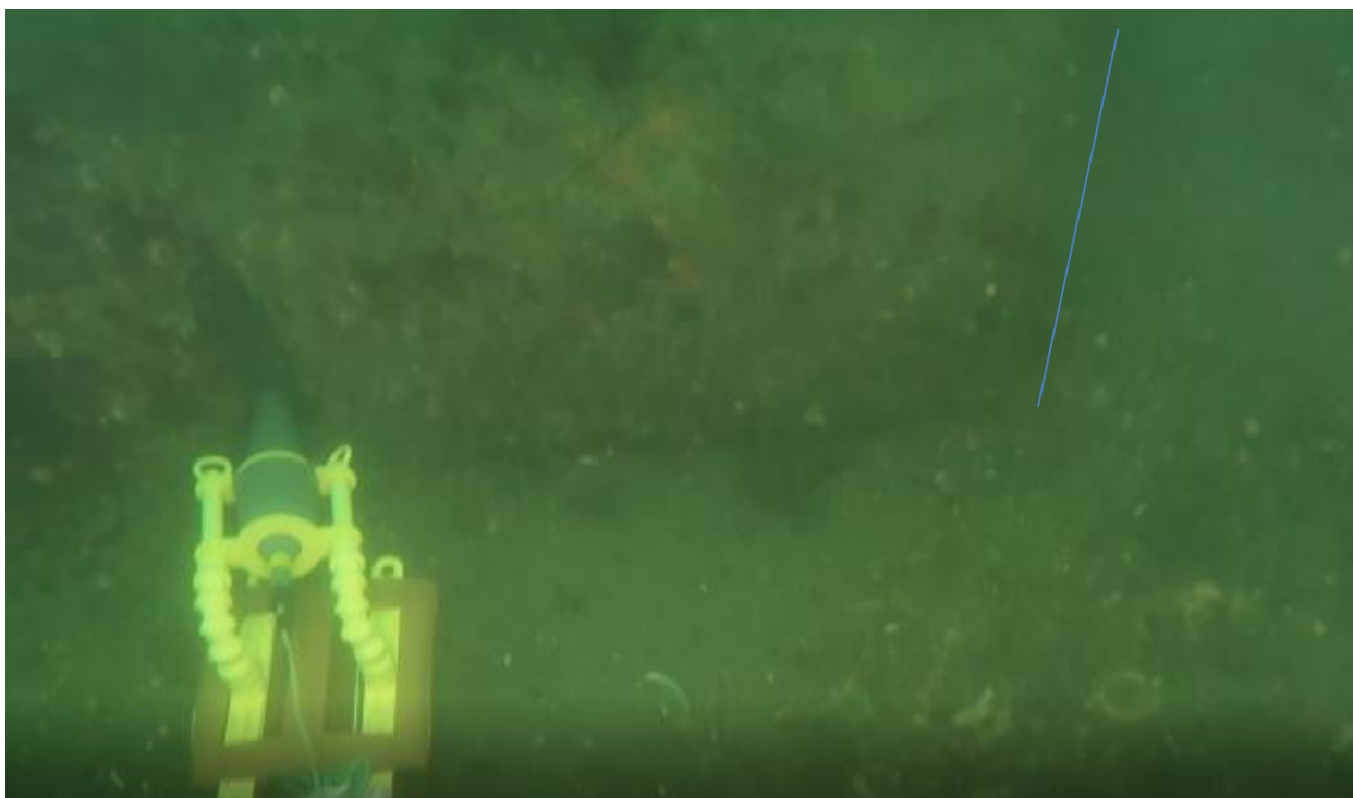
Figure 3: Mine Juliet with Pluton Shaped Charge was Position approx 500mm back from the Nose (highlighted).
