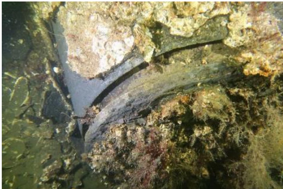
Figure 6: Mine November – Deflagration Internal Overpressure split the mine charge
