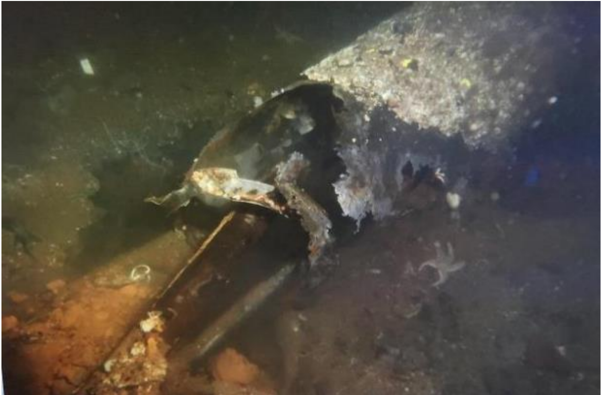
Figure 3: Deflagrated main Charge Case showing that most of the Amatol main Charge has either burned or shattered and ejected.
