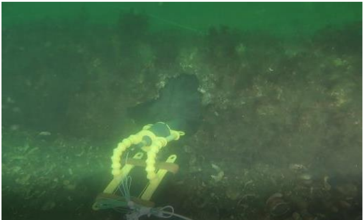
Figure 1: Mine November with Pluton Charge positioned for Low Order.
