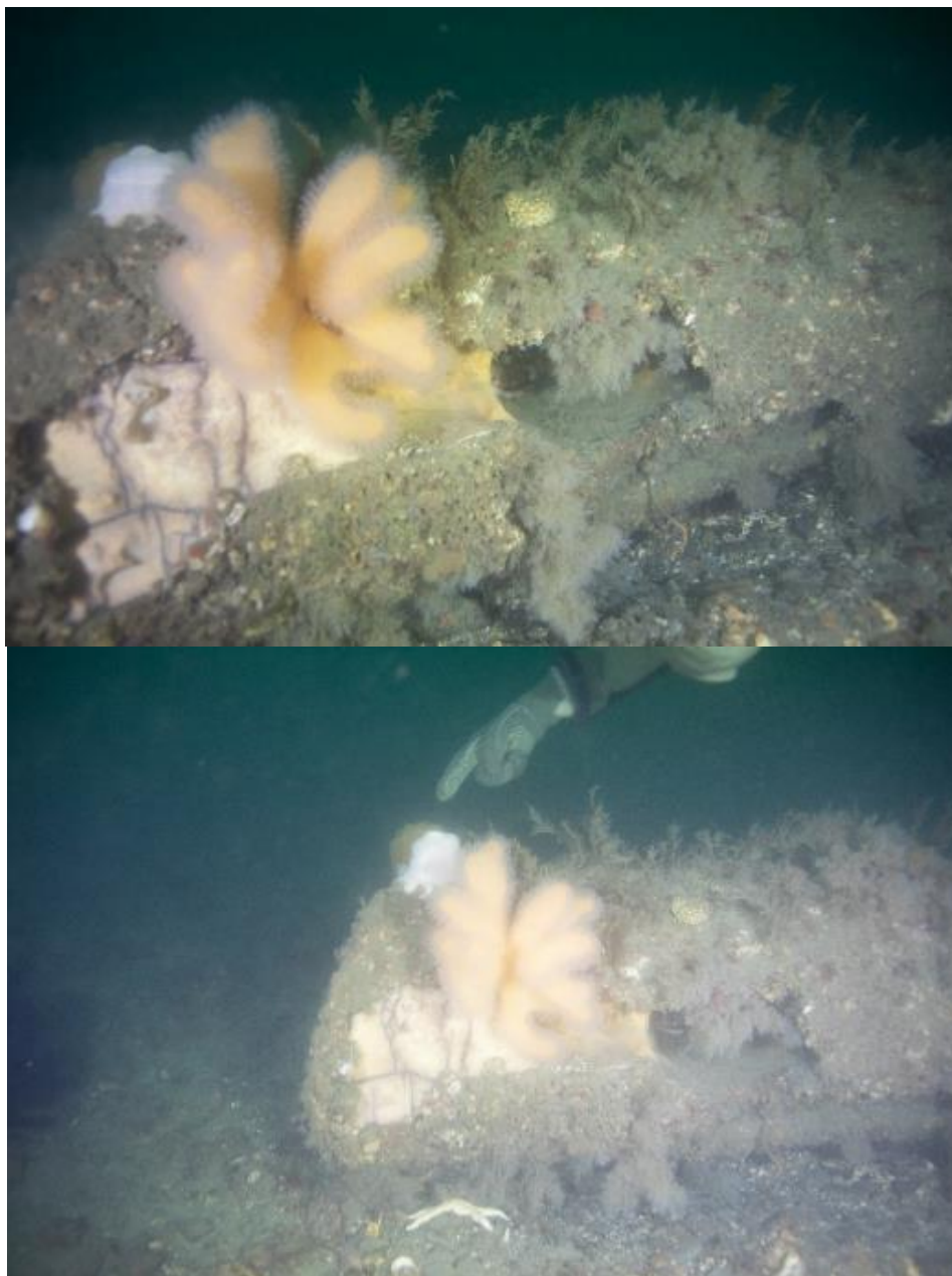
Figure 1: Mine Foxtrot Heavily Encrusted with Marine Growth. Mine Charge Case Corroded, Exposing a Brown Amatol Explosive Fill.
