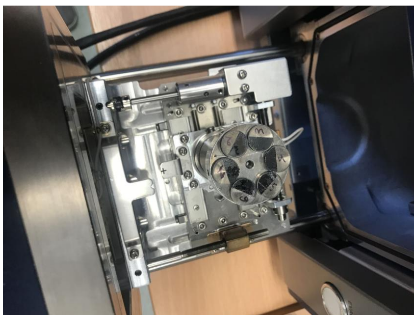
Figure 43. SEM/EDX sample holders containing samples ready for analysis
