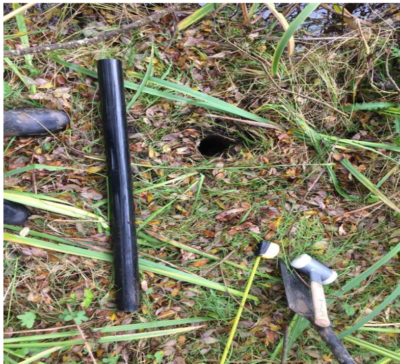
Figure 23. Sampling tools (plastic tube and mallet)
