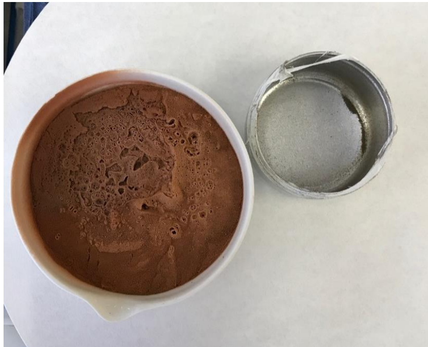
Figure 38. Example of a soil sample from Needle's Eye after LoI (left side crucible containing soil sample, right side empty aluminium pot)
