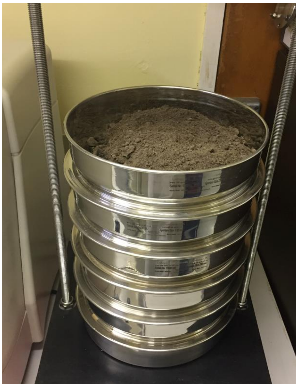
Figure 25. Sieve shaker
