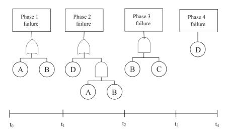
Fig. 2 Example system phased mission fault trees
