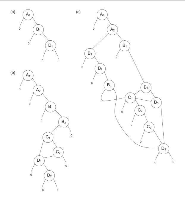
**Fig. 4** (a) BDD for phase 2 transition failure; (b) BDD for phase 3 transition failure; (c) BDD for phase 4 transition failure
