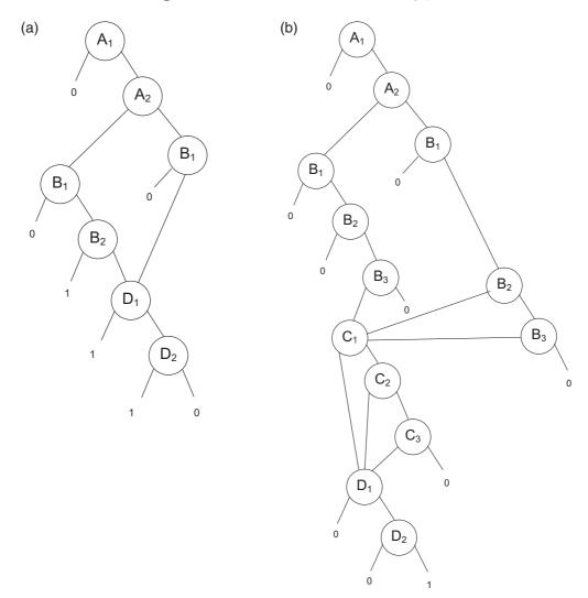
Fig. 3 (a) BDD for phase 2 failure; (b) BDD for phase 3 failure; ((c) overleaf)
