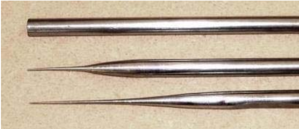
Figure 2. Manufactured rods: a reference uniform rod (above) and two tapered rods of different quadratic profiles (below).
