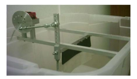
Figure 3. View of the assembled propulsion rig in a an empty water tank used for in-tank testing: the main propulsive plate made of white rubber is stiffened by two narrower plates of black rubber; holes drilled on the motor disk are used for changing amplitudes of plate vibration.
