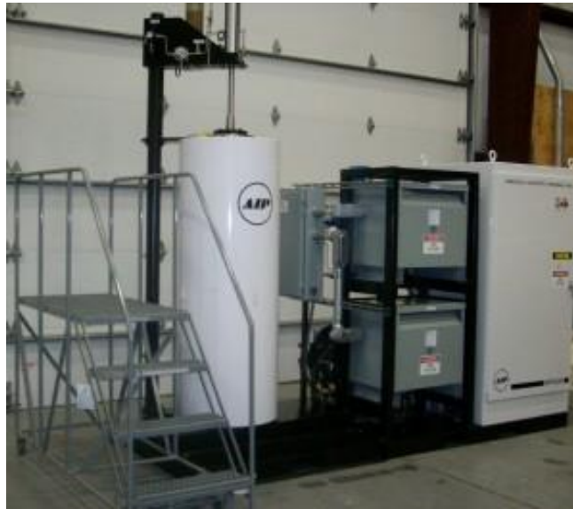
Figure 44 HIP facility used to sinter YAG samples at AIP, AIP 6-45H, Colommbus, USA
