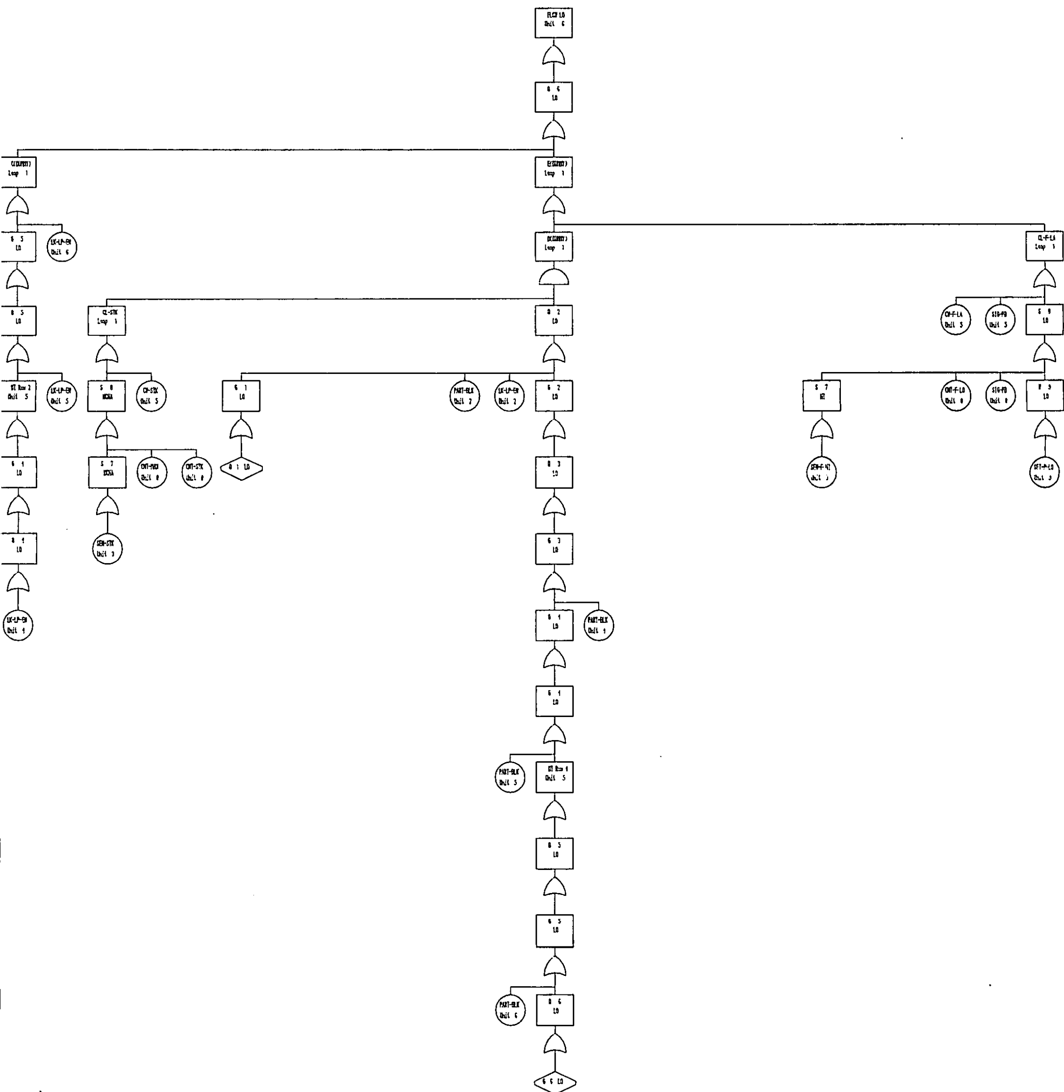
Figure 6.9 - complete fault tree for the system shown in Figure 6.1, with special control loop treatment
