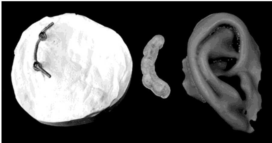
Figure 3: SLM retention bar, SLA substructure and ThermoJet wax pattern
