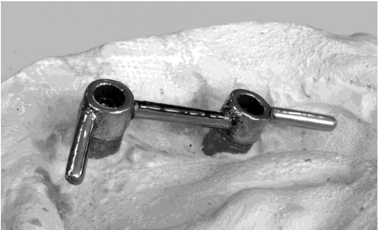
Figure 5: SLM bar fitted to patient cast
