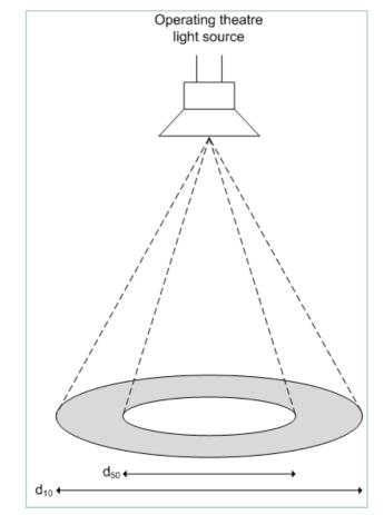
The uniformity ratio between the  $d_{10}$  and  $d_{50}$  measurements can provide an indication as to the drop off of light away from the centre of the field. It is expressed as a simple ratio indicating the relative amount of light at the two measured points. A ratio of 1 will indicate that both areas have the same amount of light which suggests a more uniform performance.
