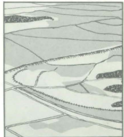
Simple mechanical shading technique using a single tone for all built-up areas.
