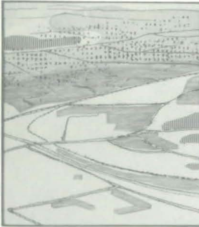
Complex mechanical shading technique using two different tones and a superimposed texture.
