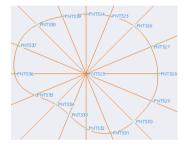
Figure 116. An illustration of sampling 16 points from the elbow cross sections
