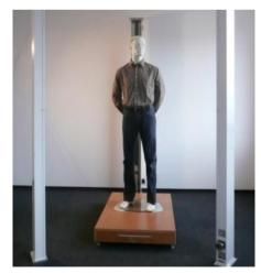
Figure 137. Vitus Smart LC (Human Solutions, 2011) 3D laser scanner
