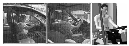
Figure 6. RAMSIS's overlay technology to fit posture and anthropometric data (adapted from Seidl (2004))
