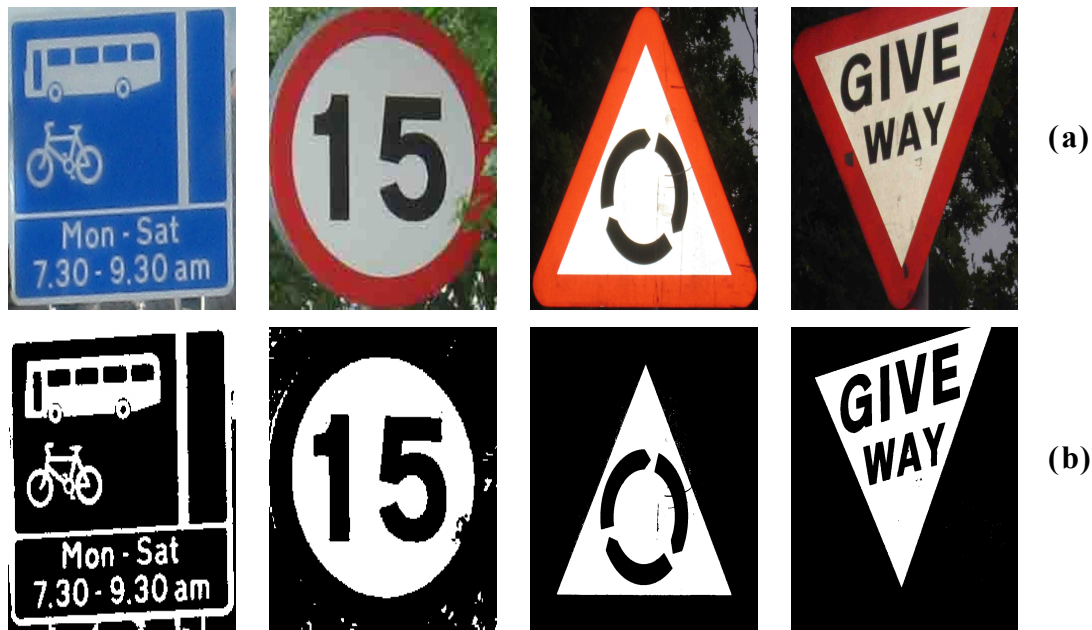
Figure 7.3: White and Black area extraction (a) Original road Sign image (b) Binary image representation
