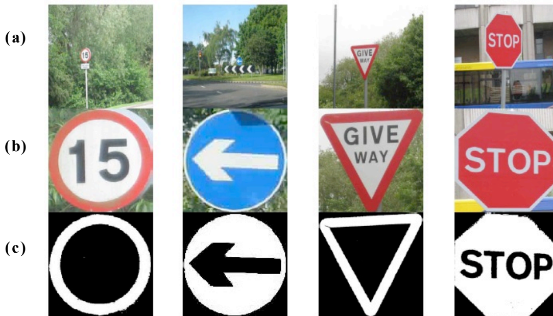
Figure 4.18: Colour segmentation using HSV colour space (a) Original Image (b) Cropped road sign from original image (c) Cropped road sign from binary image
