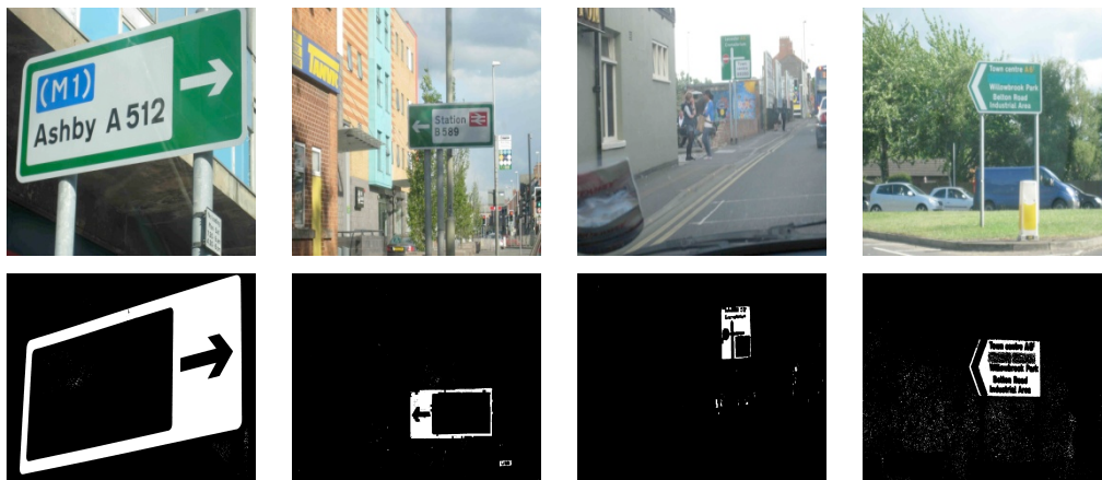
Figure 5.9: Segmentation of Green colour Road Signs
