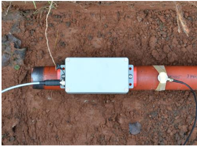
Figure 8.7. Source generator coupled to the pipe
