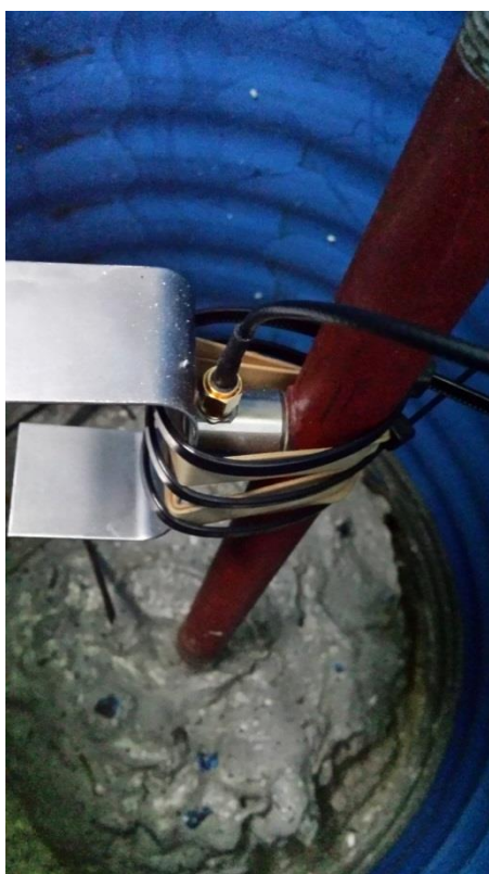
Figure 4.39. Photograph of transducer coupled to protruding waveguide at Nafferton
