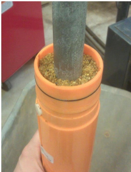
Figure 8.24. Photograph of active waveguide physical model employing an inclinometer casing, with Leighton Buzzard sand backfill and 25 mm diameter steel waveguide tube
