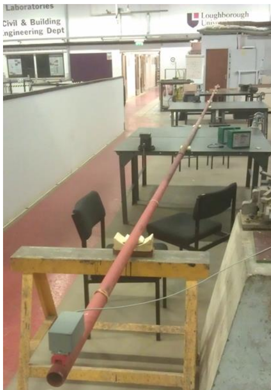
Figure 8.1. Photograph of experimentation to measure attenuation in an air-waveguide-air tri-layer system
