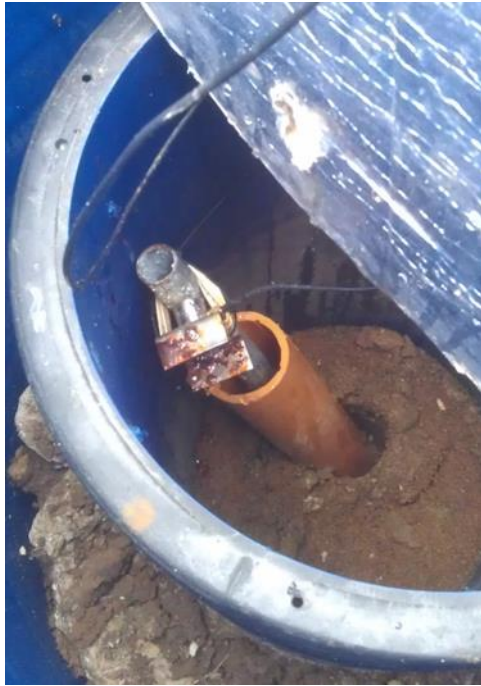
Figure 4.5. Deformed retrofitted inclinometer at Hollin Hill (AEWG In2)
