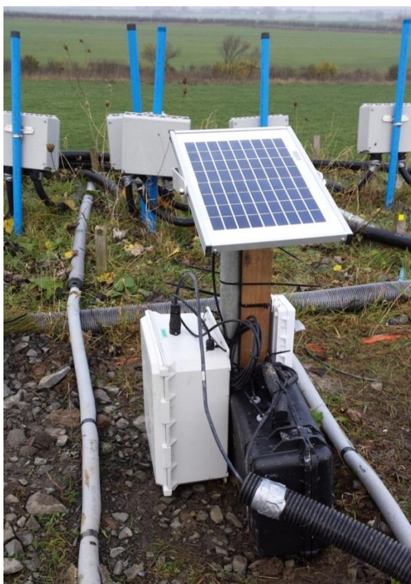
Figure 4.41. Photograph of SAA data logger and solar panel, and Slope ALARMS batteries at the top of the slope at Nafferton
