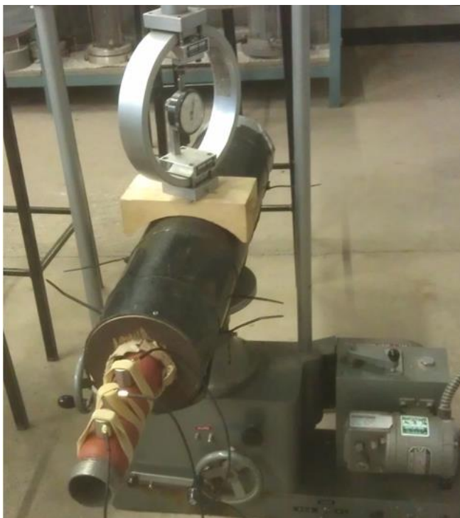
Figure 6.4. Photograph of the active waveguide model installed in the Dixon & Spriggs (2007) constant strain rate compression apparatus
