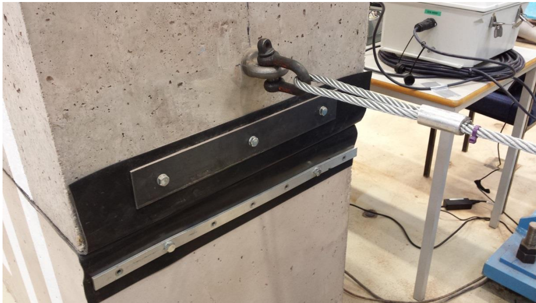
Figure 7.4. Photograph showing the wire rope fastened to the resin anchor at the front face of the top block. Geomembrane interface fixings are also shown
