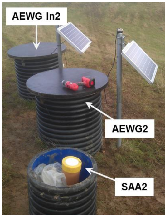
Figure 4.4. Photograph of instrumentation installation at Cluster 2 at Hollin Hill: surface covers of AEWG In2, AEWG2 and SAA2
