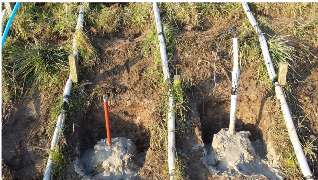
Figure 4.38. Photograph of active waveguide and SAA installations (both grouted) at Nafferton
