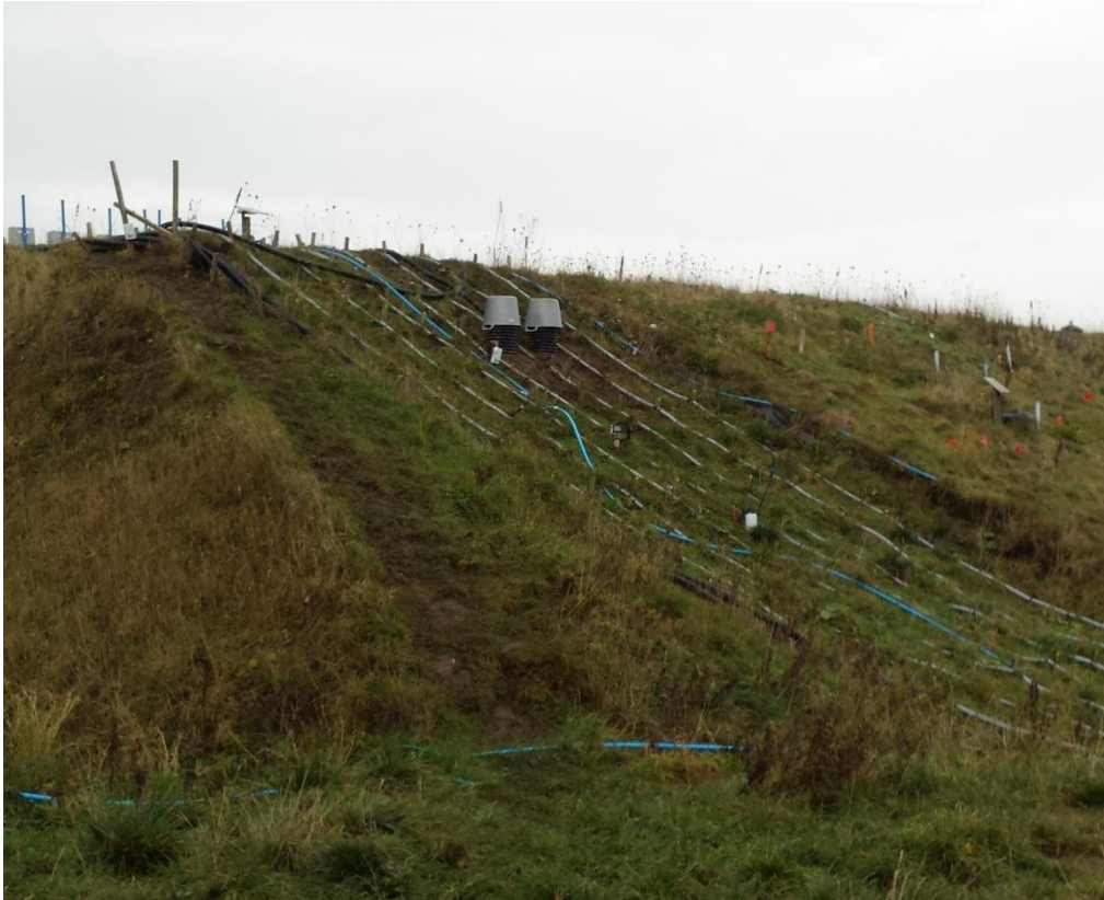
Figure 4.42. Photograph of Slope ALARMS and SAA surface covers on the slope at Nafferton
