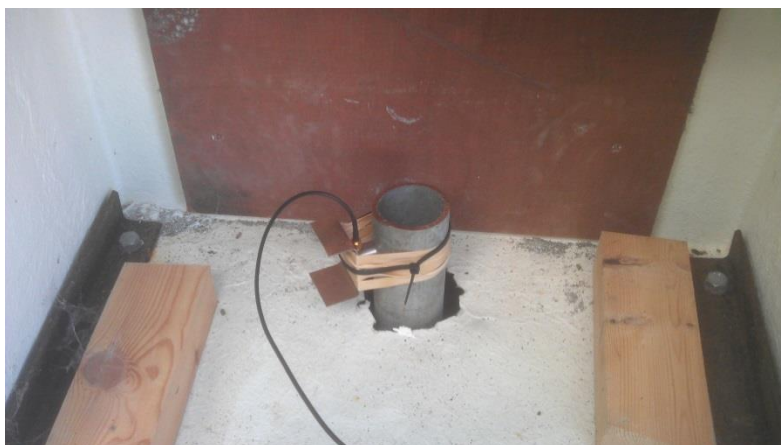
Figure 4.28. Photograph of instrumentation installation at Scarborough Spa: waveguide with transducer attached
