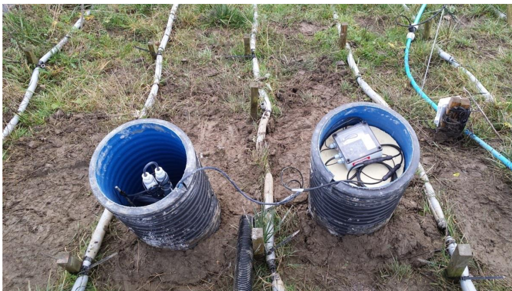
Figure 4.40. Photograph showing SAA and Slope ALARMS protected by surface covers at Nafferton
