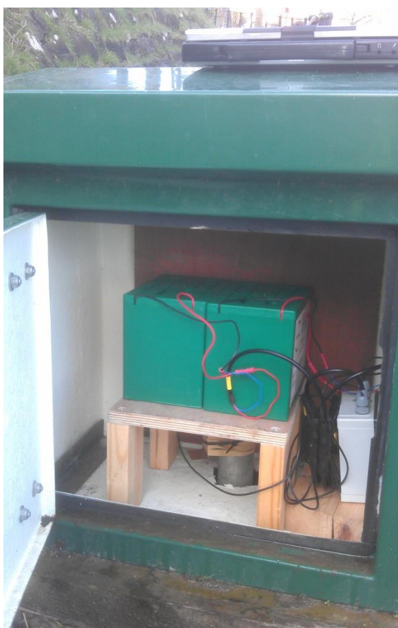
Figure 4.29. Photograph of instrumentation installation at Scarborough Spa: sensor and batteries inside surface cover
