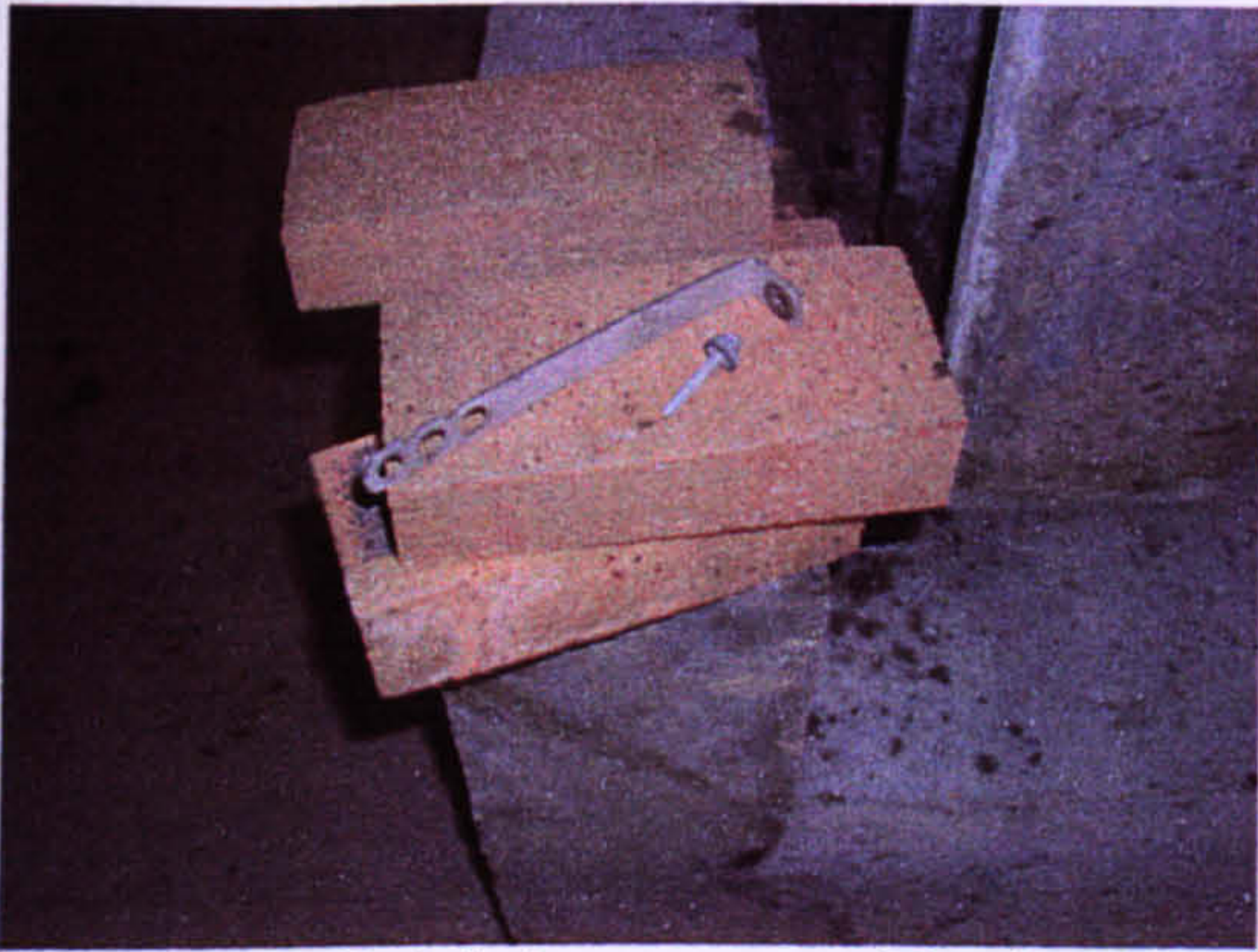
The rivet and brick tie
