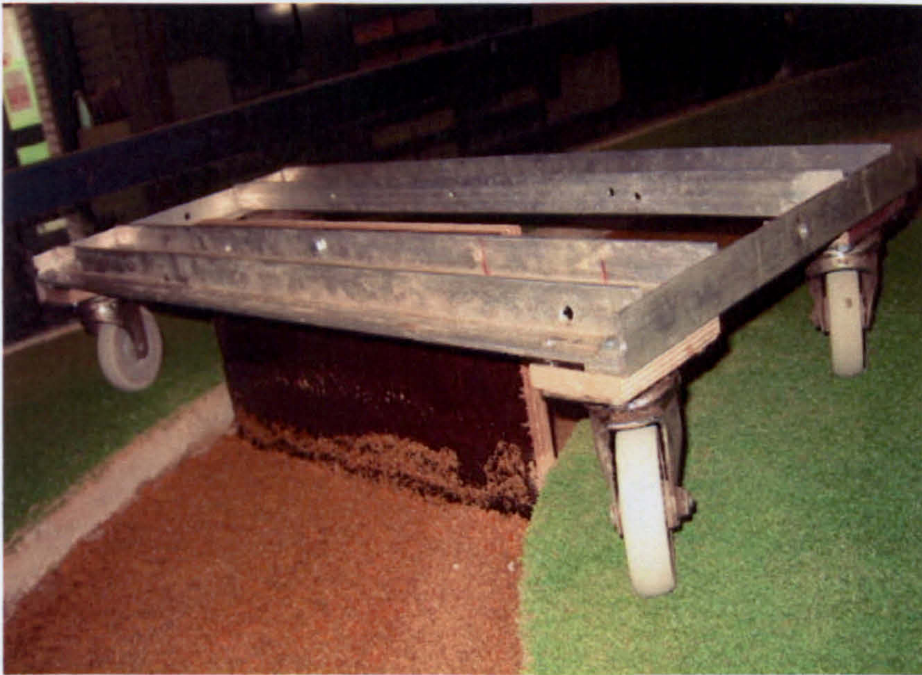
Figure 3.10: Plywood board attaching to an aluminium frame with roller for screeded sand
