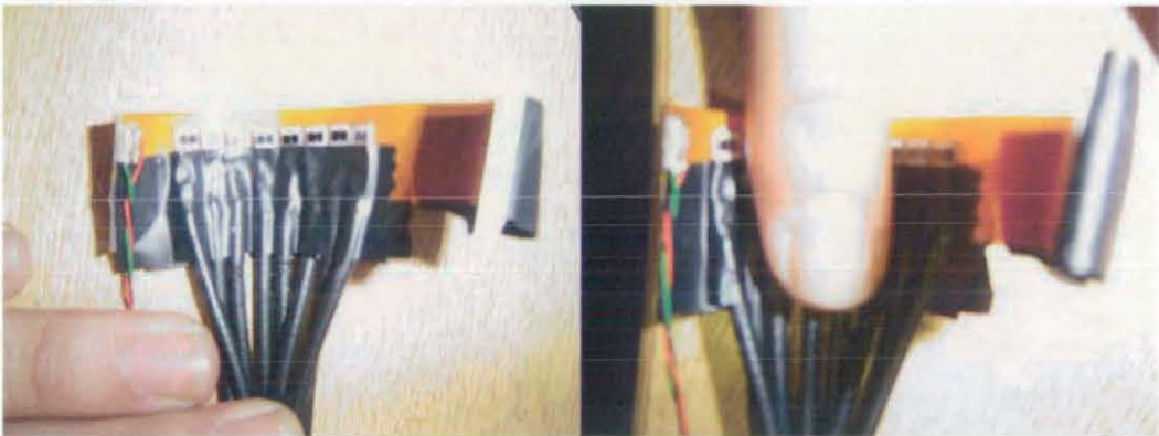
Figure 4.9 - Photodiode array solution for recording transmitted intensity distributions. Photodiode array ring sensor with dual wavelength light source (left) and finger placement prior to securing (right).
