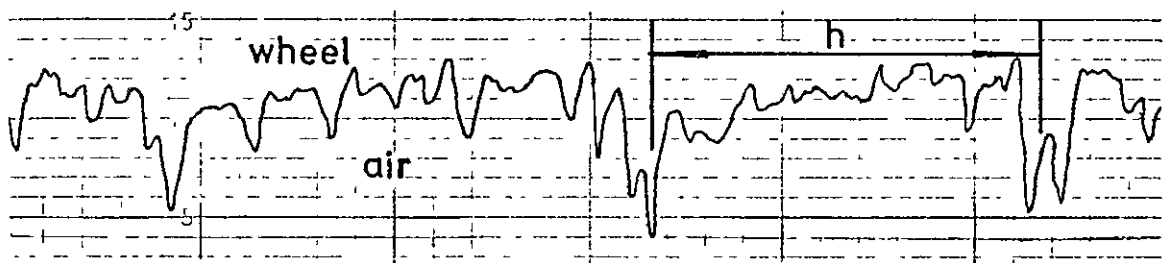
Test N o 5 Wheel type:- A 60 KV R_a = 1.30 \mu\text{m}
