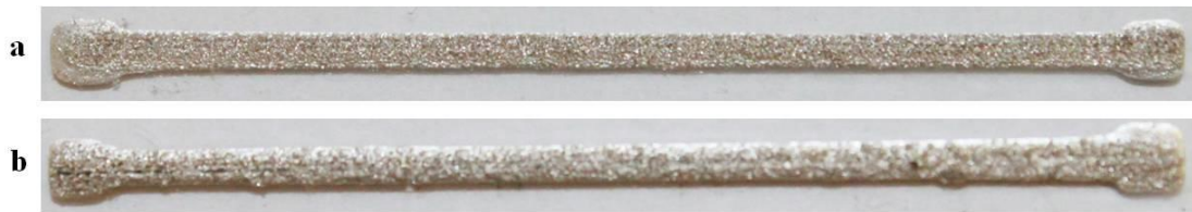
Figure 5.15: Direct comparison between an undamaged track (a) P-2.3-1 and damaged track (b) P-3.1-1
