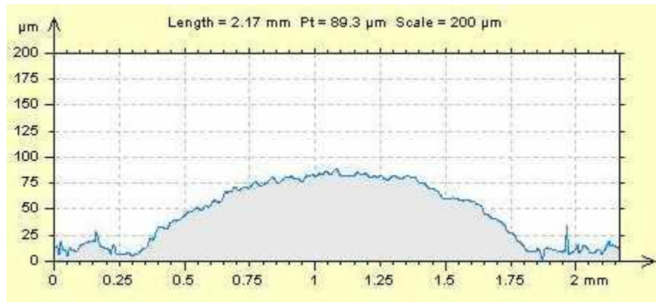
Figure 5.8: the cross-section profile of oven cured sample at 150^{\circ}\text{C} for 0.5\text{h}
