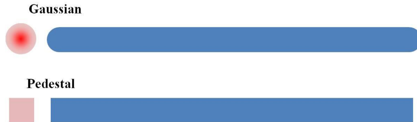
Figure 6.6: The edge effect of beam shape during a single track scan
