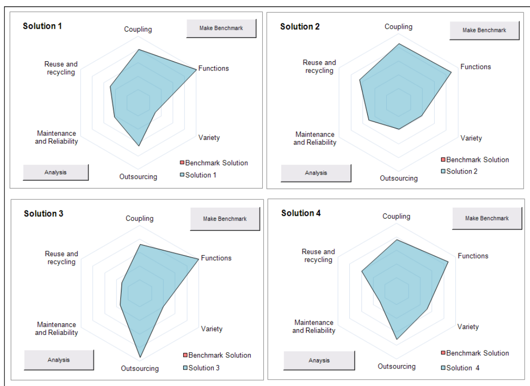
Figure 8.14. Optimal solutions for the automotive climate control system with the focus on technical modularity
