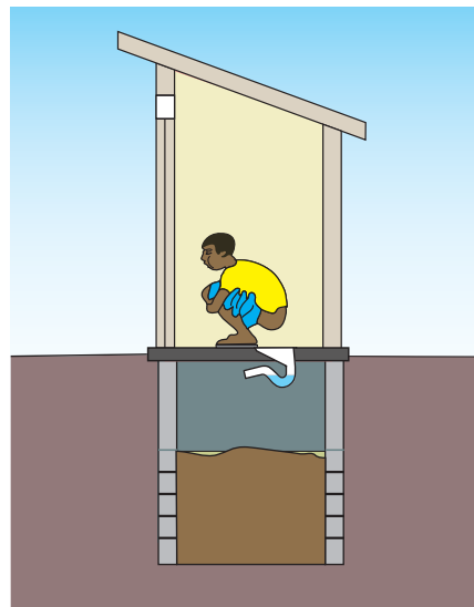
Figure 3. A direct pour-flush latrine
