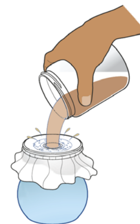
Figure 33. Straining water through a fine mesh cloth
